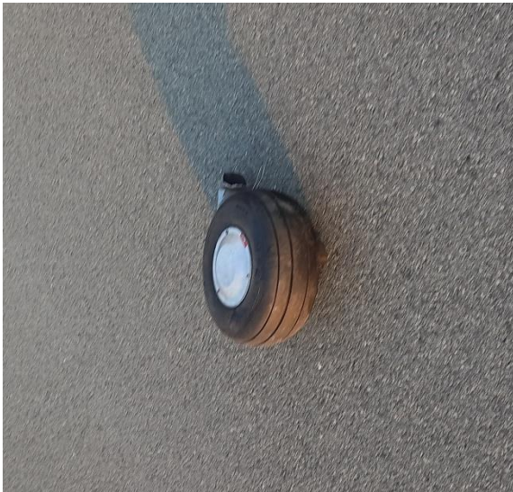
Fig. 2. Separated wheel of the main landing gear (source: PKBWL)
