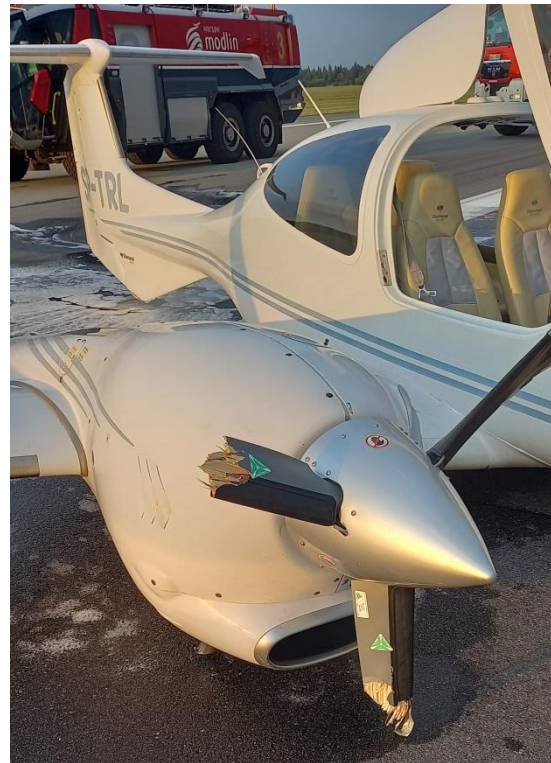
Fig. 3. Damaged propeller of the right engine (source: PKBWL)
