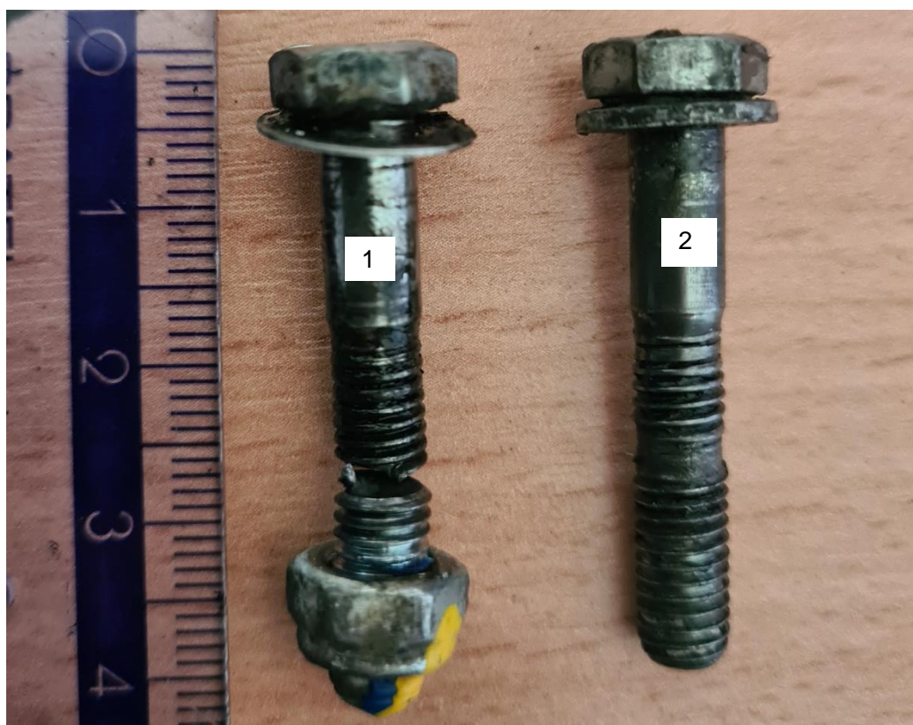
Fig. 1. Broken (1) and damaged (2) bolt of the stabilator hinge [source: PKBWL]
