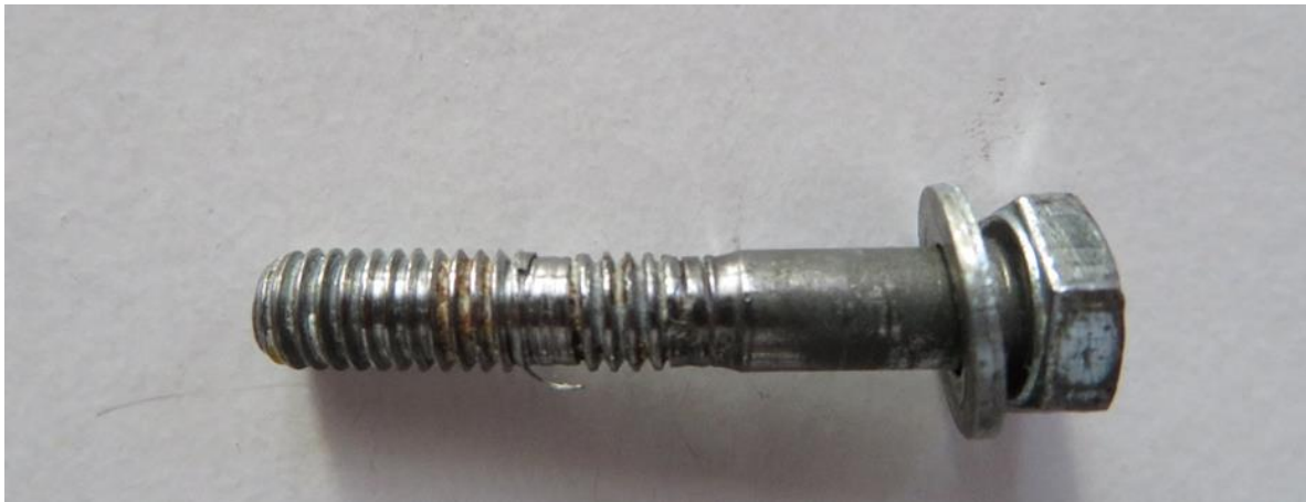
Fig.3. The right bolt with damaged thread [source: PKBWL]
