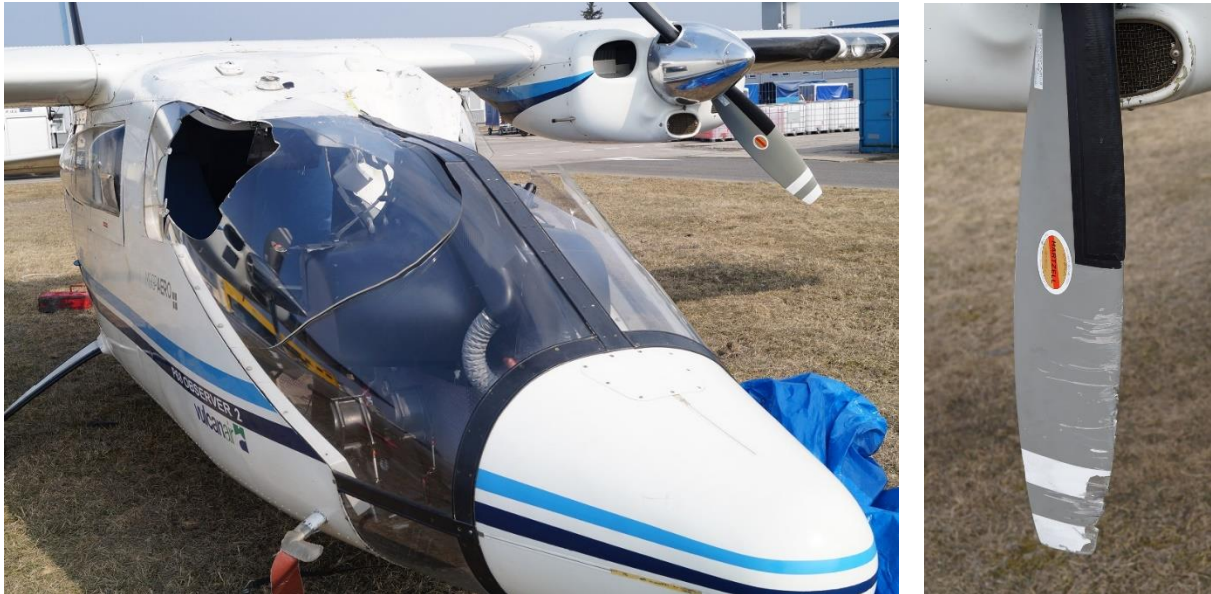
Fig. 1. VULCANAIR P68 airplane: damaged cockpit glazing (left photo) and damaged RH propeller blade (right photo) [source: PKBWL]
