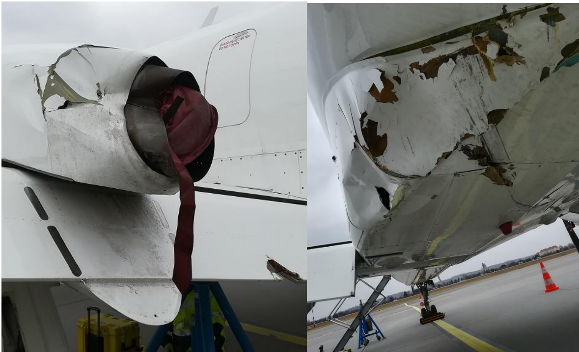
Fig. 4. SAAB-340A airplane: L/H engine and L/H wing flap damages (photo at left) and lower fuselage part (photo at right) [source: Gdańsk Airport]
