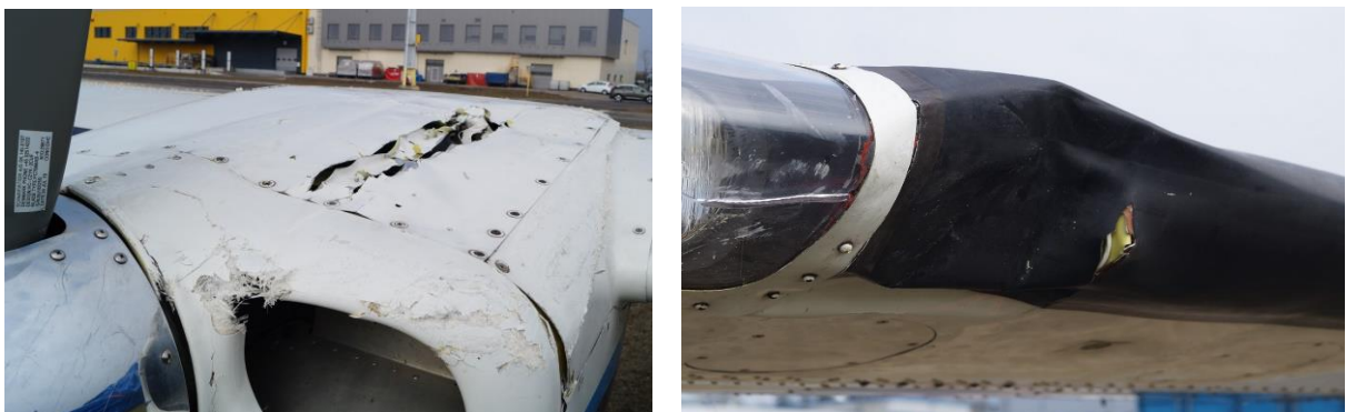
Fig. 2. VULCANAIR P68 airplane: damaged RH engine cowling (left photo) and damaged LH wing (right photo) [source: PKBWL]
