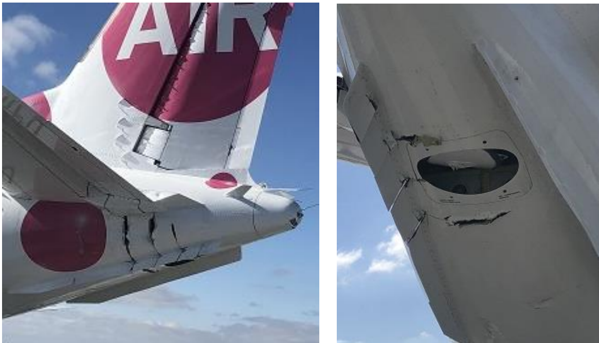
Fig. 3. SAAB-340A airplane rear fuselage part damages [source: Gdańsk Airport]
