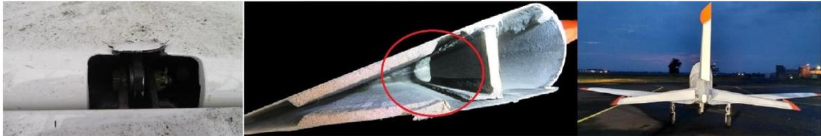
Fig. 6. The horizontal tail hinge mounting hole, jack end and tail angle [source: PKBWL, test pilot]
