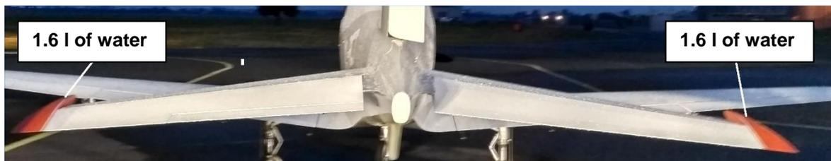
Fig. 7. Amount of water that was poured into the elevator [source: PKBWL, test pilot]
