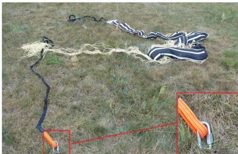
The parachute with the rocket engine was found 43.5 m from the tail of the plane. The shackle connecting the system with the airframe was closed.
