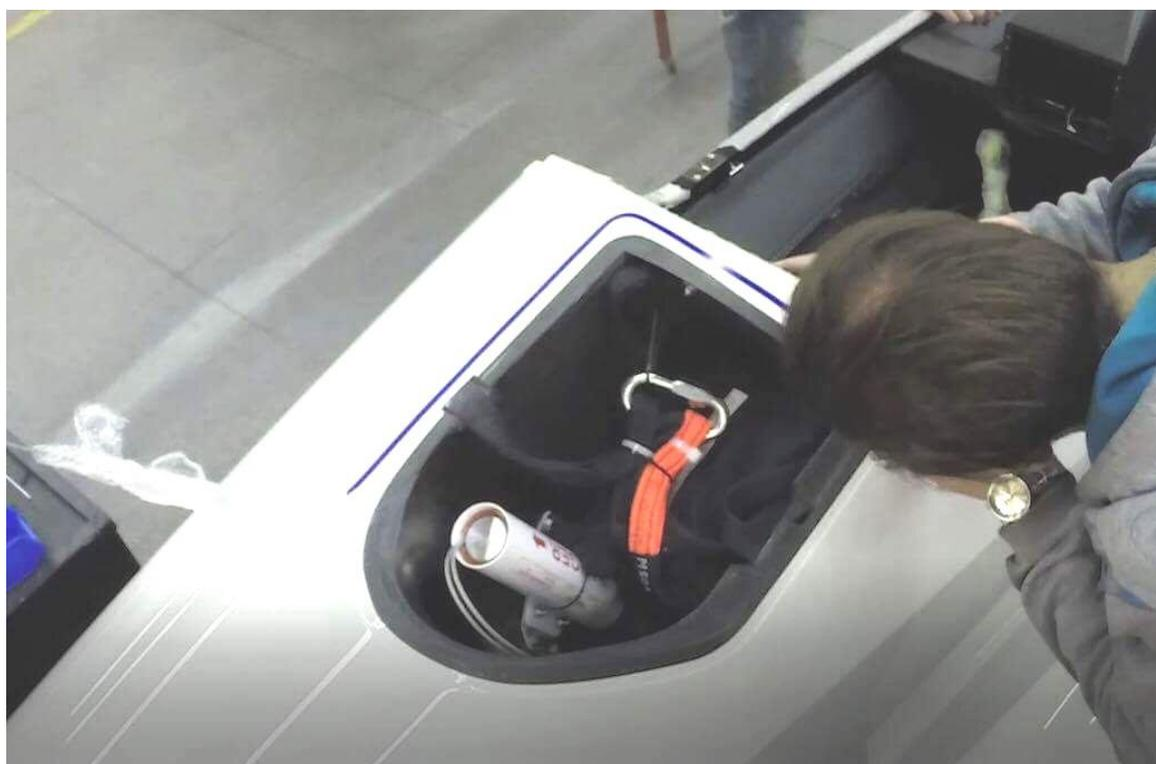
Fig. 9. Ballistic Recovery System installed on a Tarragon aircraft [source: SIA Pelegrin]
