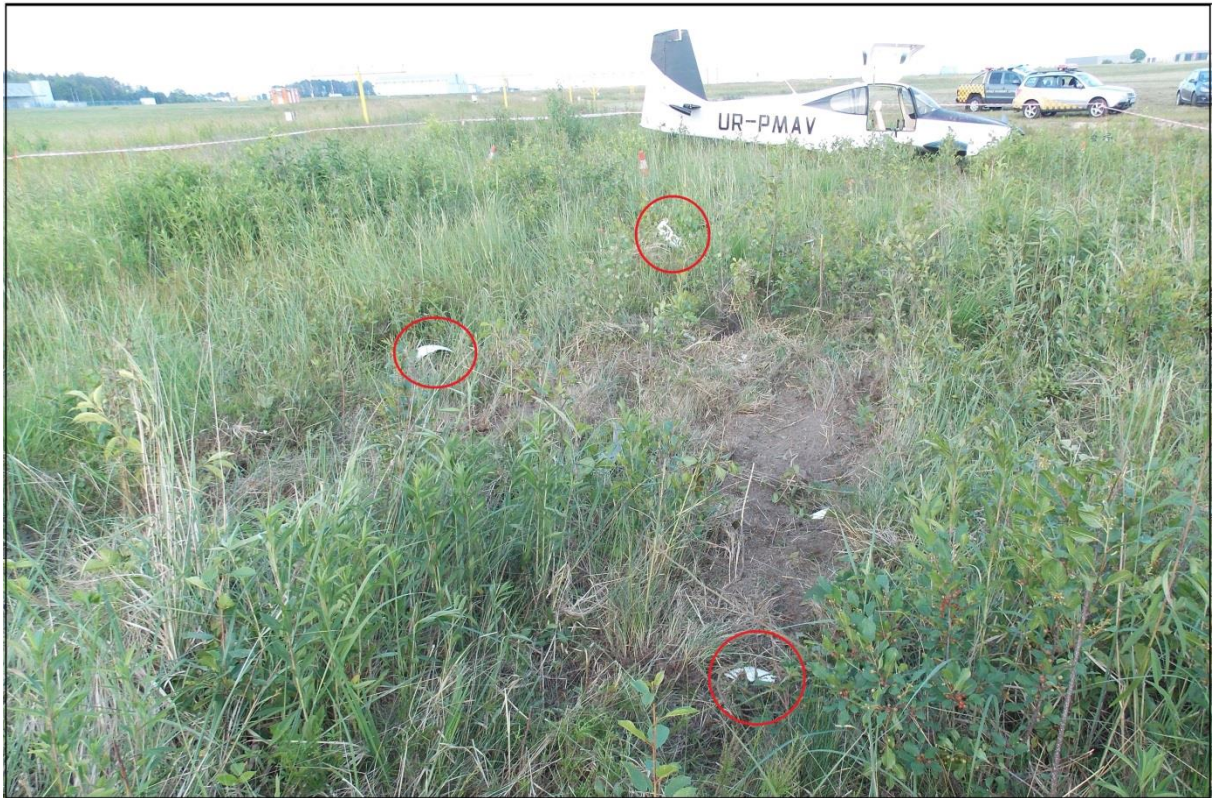
Fig. 11. Touchdown marks and fragments of the landing gear fairings [source: PKBWL]
