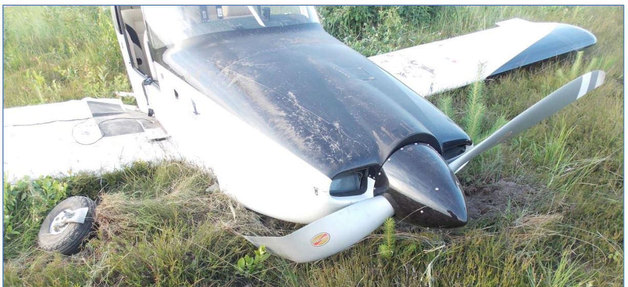
Fig. 10. Separated nose wheel and bent propeler blade. [source: PKBWL]
