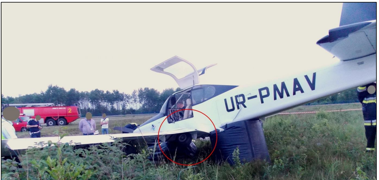
Fig. 6. Damaged airplane - left side view. Visible damaged the left main landing gear and left wing. [source: PKBWL]
