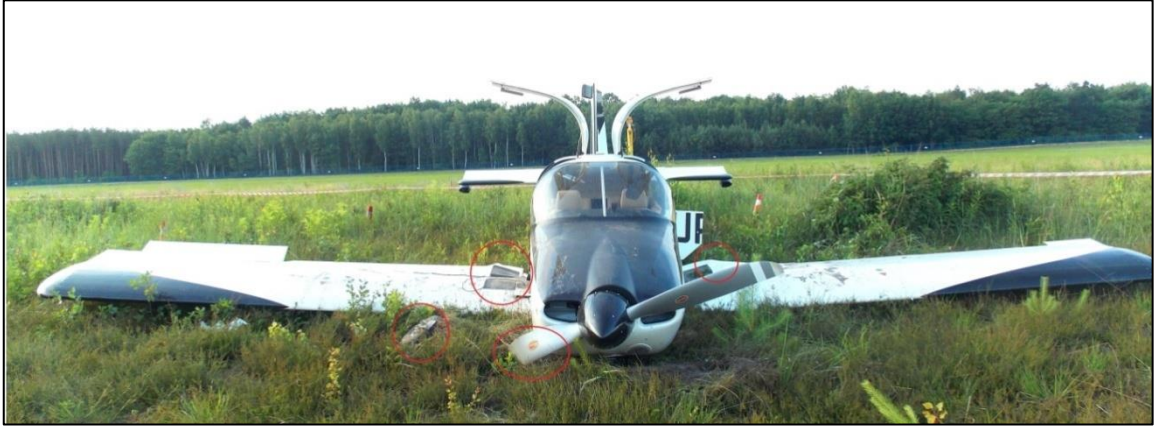
Fig. 4. Damaged airplane - front view. Visible damaged propeller, wings and separated nose landing gear. [source: PKBWL]
