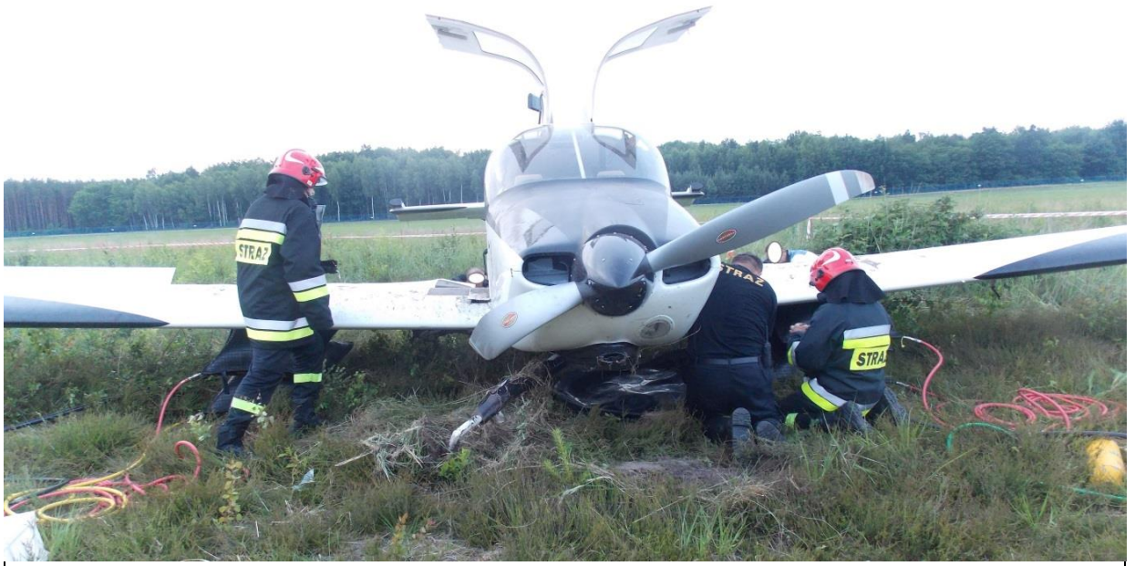
Fig. 14. Fire brigade in the course of emptying the left tank. [source: PKBWL]
