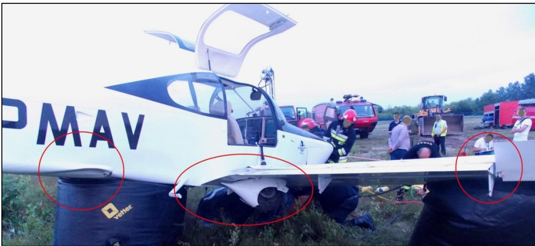
Fig. 5. Damaged airplane – right side view. Visible damaged right main landing gear, right wing, lower part of the fuselage and broken aileron. [source: PKBWL]
