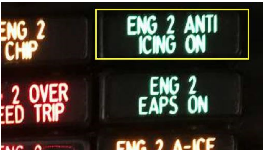
Figure 27: Operation light ENG 2 Anti-Icing ON
