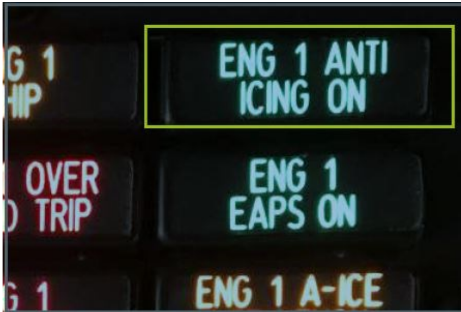
Figure 26: Operation light ENG 1 Anti-Icing ON
