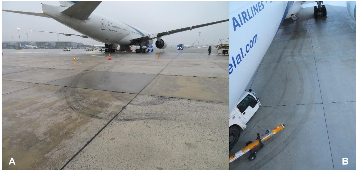
Fig. 10. EPWA apron: A – marks of the right truck of the main landing gear wheels; B – marks of the front landing gear wheels
