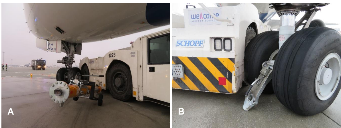
Fig. 9. Occurrence site: A – general view showing the positions of the aircraft, towbar and the tractor after the occurrence; B – collision of the nose landing gear with the tractor
