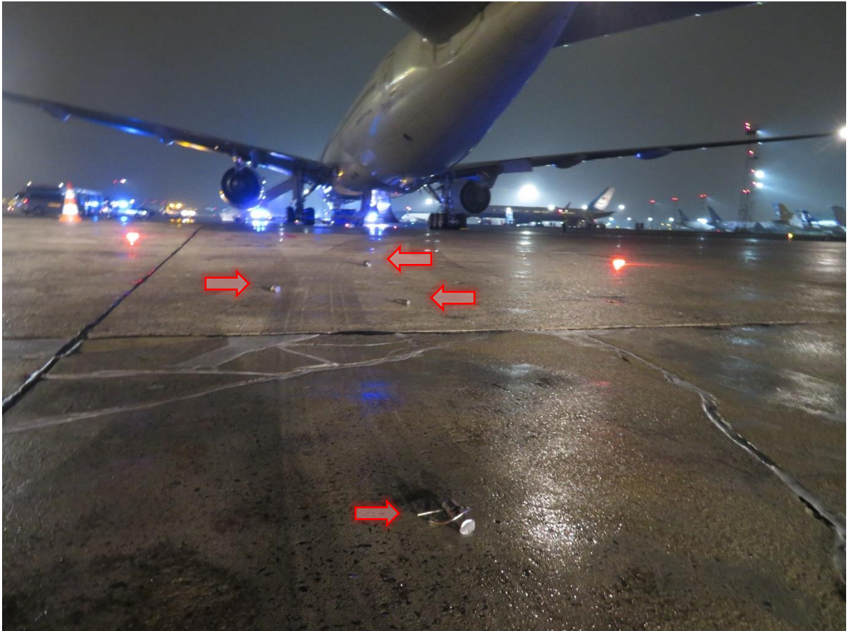
Fig. 5. EPWA aerodrome apron – the arrows show the fragments of the left shear pin (relative to the direction of the tractor-aircraft combination movement)
