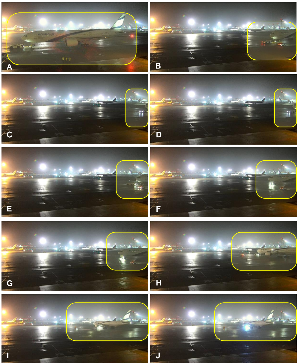
Fig. 1. Boeing B777-258, accident aircraft, during push-back and towing: A – push-back initiation; B – right engine start-up initiation; C – end of push-back; D – towing initiation; E – end of right engine start-up; F – left engine start-up initiation; G – shearing the left pin of the towbar; H – end of left engine start-up; I – tractor being pushed by the aircraft; J – collision (aircraft and tractor stopped)
