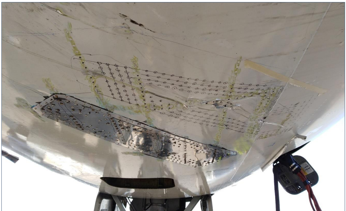
Fig. 3. B777-258, accident aircraft during repair at EPWA aerodrome – damage view
