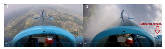
Fig. 8. Incipient spin [source: the owner of the aeroplane]
