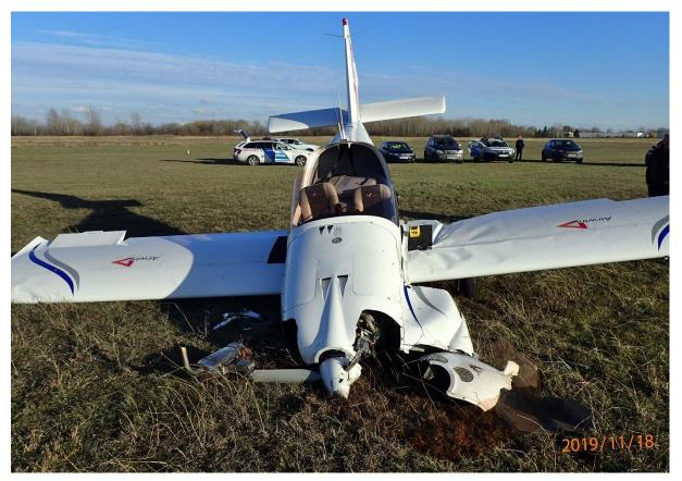
Figure 2: Visible damages to the aircraft
