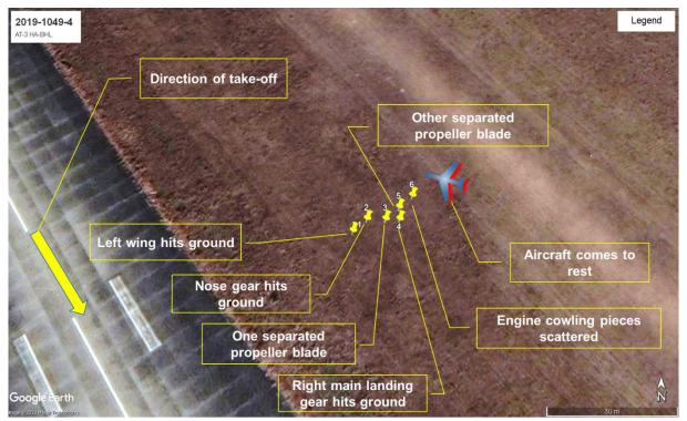
Figure 4: Locations of the marks in the ground
