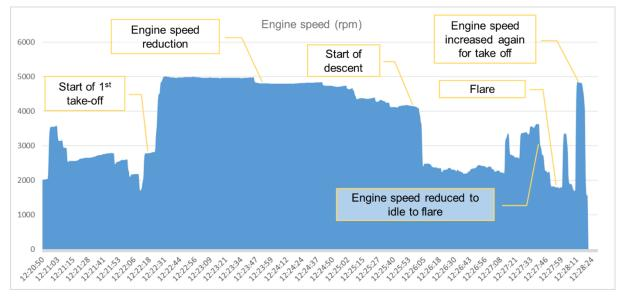
Figure 5: Engine speed diagram as a function of time during the flight ending up in the accident
