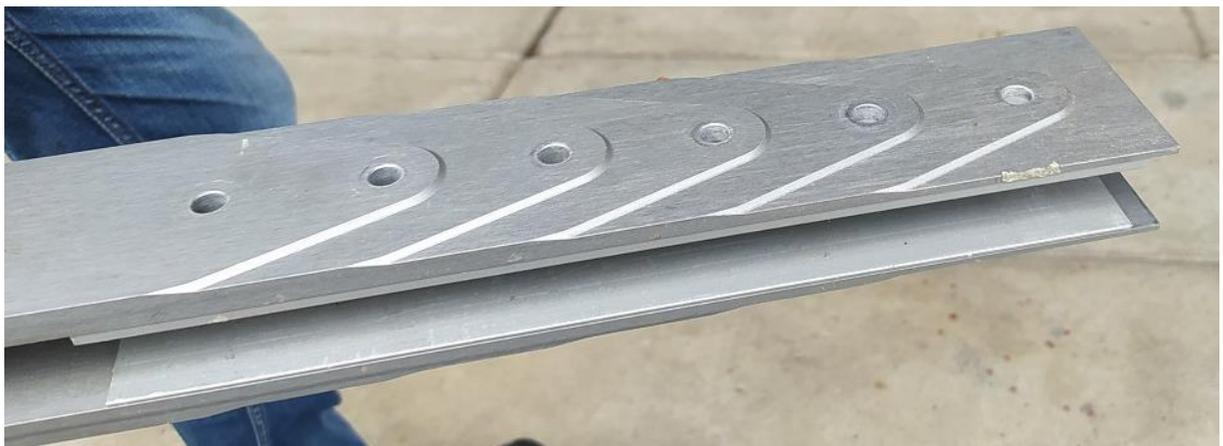
**Fig. 28.** Example of a gyroplane rotor blade connector with gradual change of its stiffness by changing its thickness [source: PKBWL]
