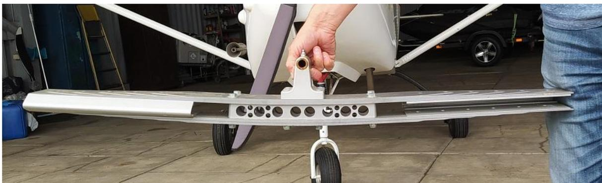
**Fig. 31. Example of a gyroplane rotor blade connector with dihedral reducing the bending moment acting on working blades [source: PKBWL]**
