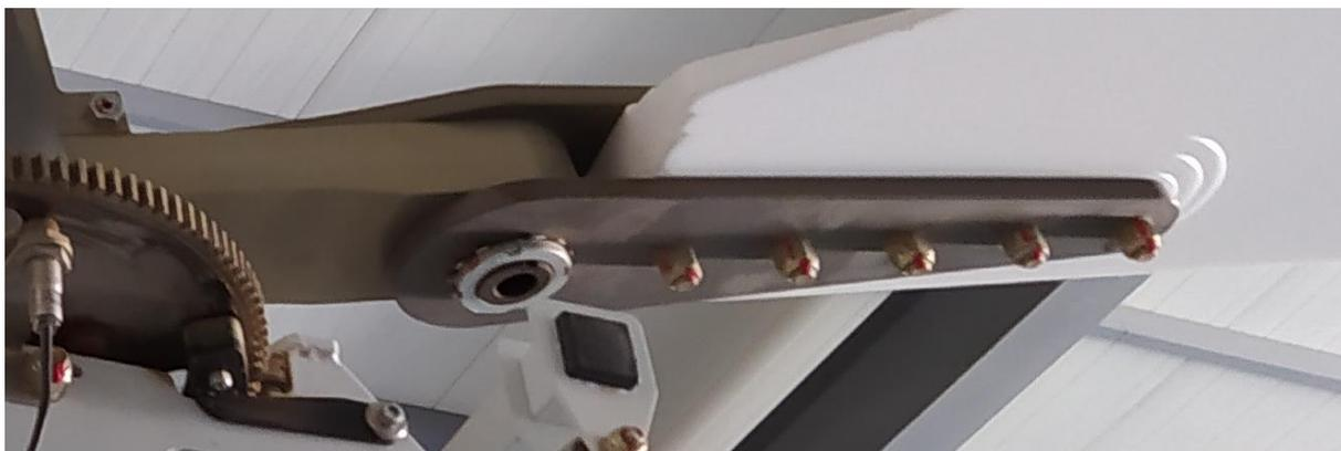
**Fig. 30. Example of a gyroplane rotor blade connector with gradual change of its stiffness by changing its width [source: PKBWL]**
