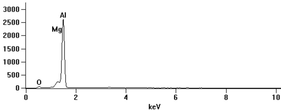
Fig. 24. X-ray microanalysis of the rotor blade chemical composition [source: Silesian University of Technology]
