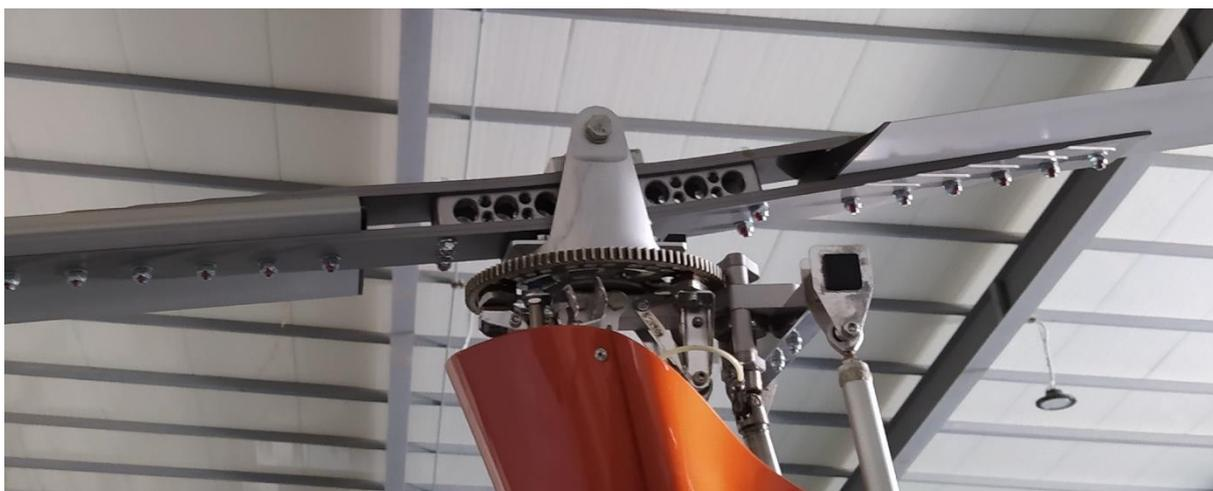
**Fig. 32. Example of a gyroplane rotor blade connector with dihedral reducing the bending moment acting on working blades [source: PKBWL]**
