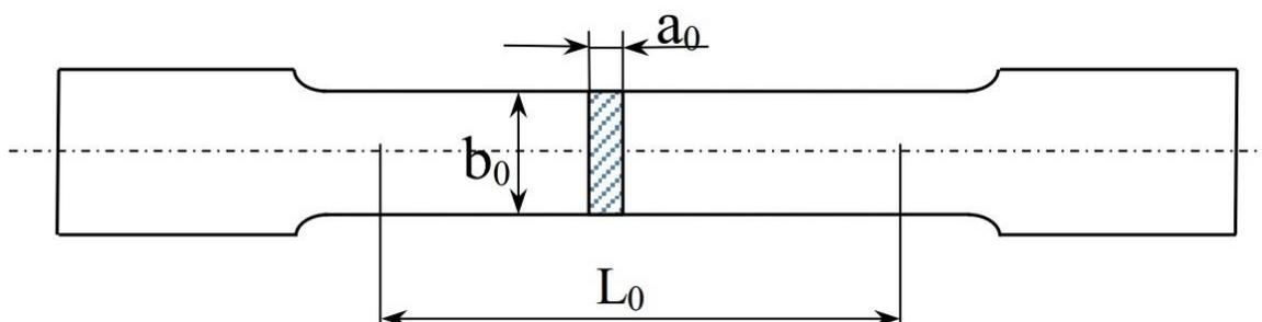
Fig. 25. A flat sample with the heads for static tensile test [source: Silesian University of Technology]
