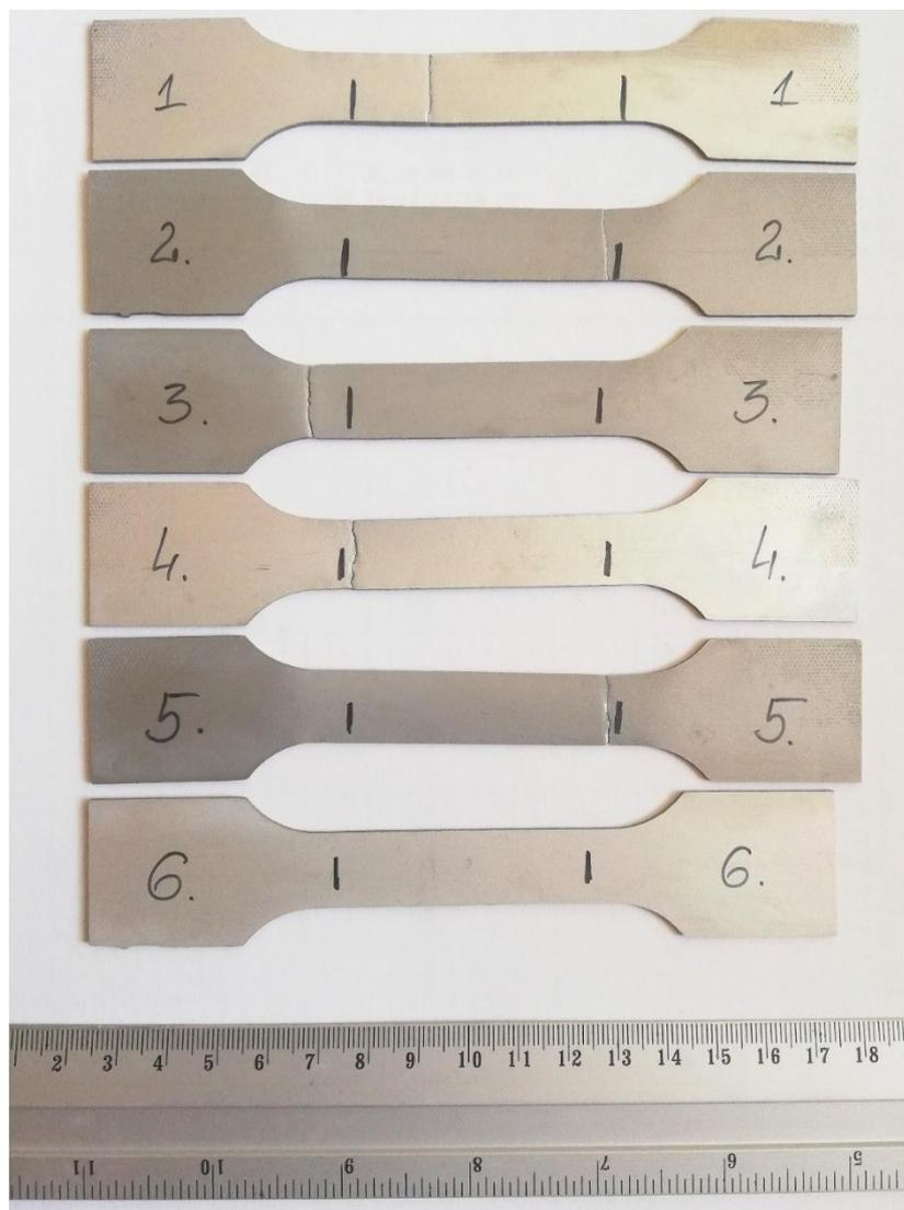
**Fig. 26. Test samples after the static tensile test. „1” to „5” – tested samples; „6” - reference sample [source: Silesian University of Technology]**
