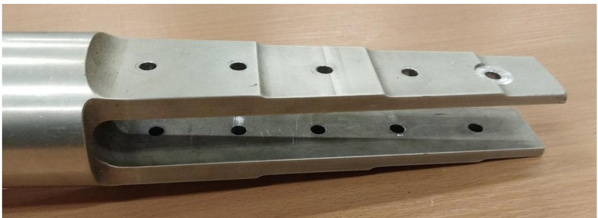
**Fig. 29.** Example of a gyroplane rotor blade connector with gradual change of its stiffness by changing its thickness [source: PKBWL]
