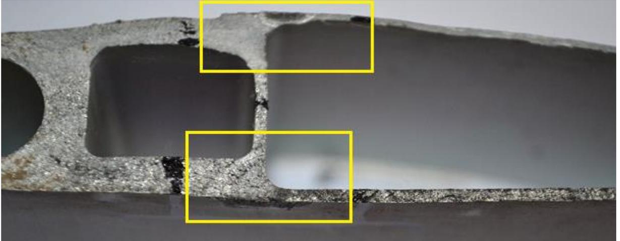
**Fig. 19. Sampling areas for examination with the scanning electron microscope [source: Silesian University of Technology]**
