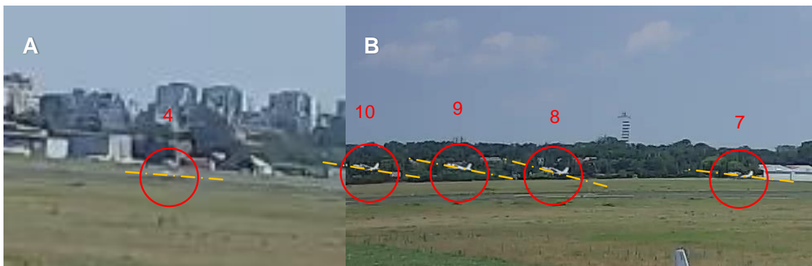
Fig. 15. Take-off of SOCATA MS 893 E-D D-EGET dated 28 June 2020 – close-up of selected shots from Fig. 14. (the orange line shows the longitudinal axis of the plane)
