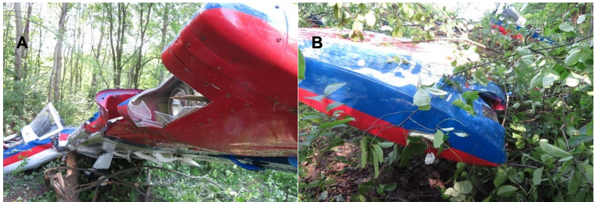
Fig. 3. SOCATA M.S. 893 E-D D-EGET aircraft, wing damage: A – left wing, B – right wing
