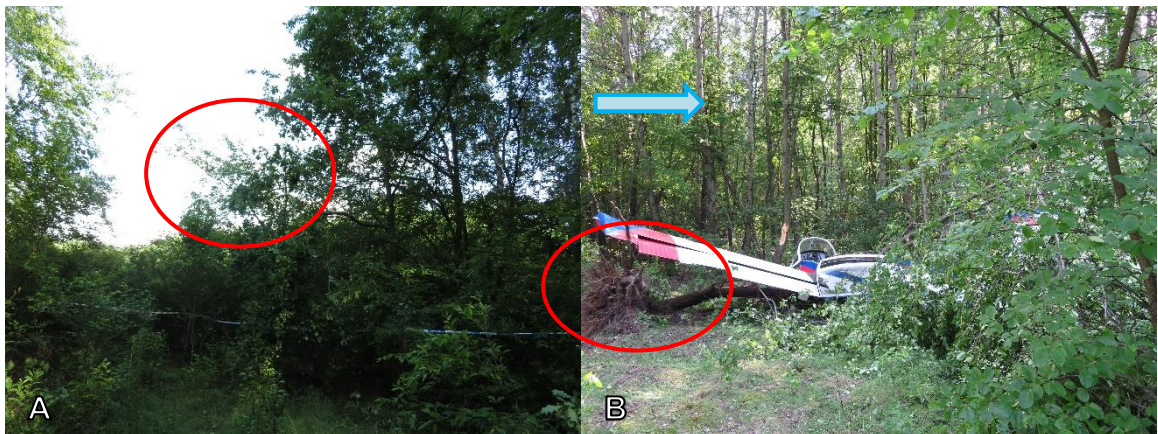
Fig. 11. Crash scene of SOCATA M.S. 893 E-D D-EGET: A – broken tree branches on the west side of forest clearing (direction opposite to the flight direction), B – overturned tree and the wreck (blue arrow shows the flight direction)
