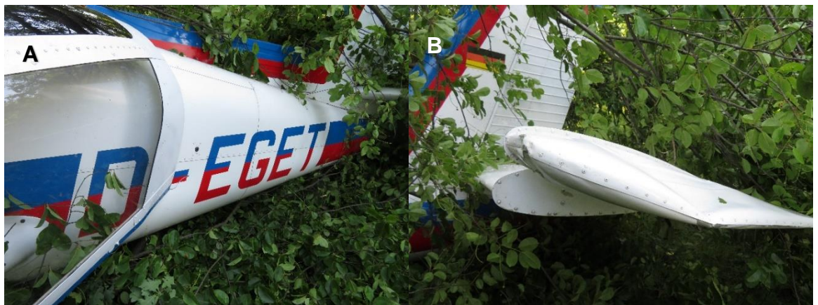
Fig. 4. SOCATA M.S. 893 E-D D-EGET after the crash: A – tail with German registration marks, no visible damage, B – empennage with visible dents
