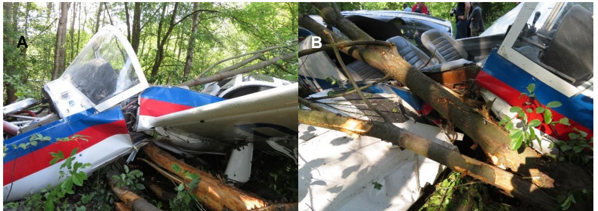
Fig. 2. SOCATA M.S. 893 E-D D-EGET aircraft, damage to the cabin: A – view from left, B – view from right
