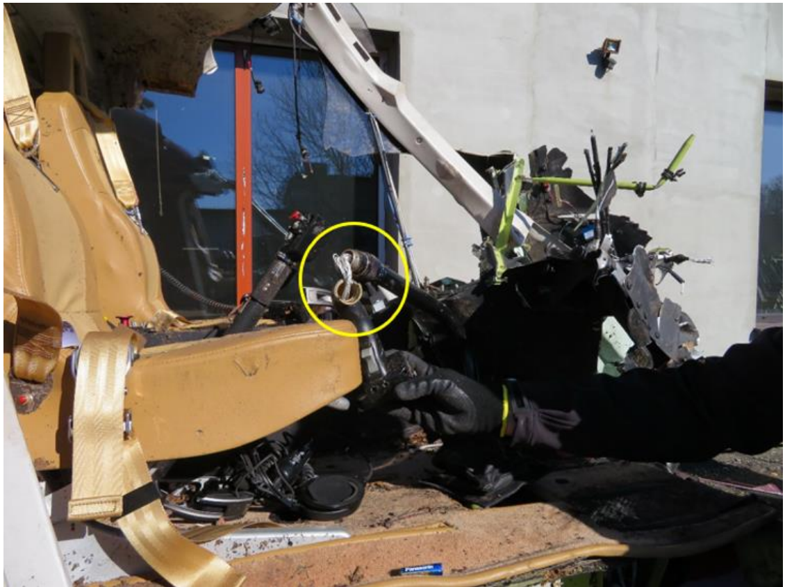
Fig. 26. Pilot's seat: visible, broken control stick, marked with a yellow circle. [source: PKBWL]
