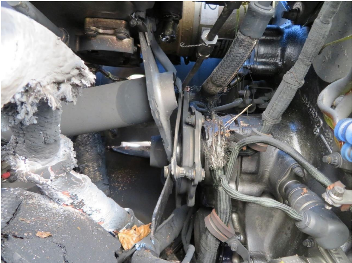
Fig. 23. Signs of local fire in the area of the left engine - view after the engine cowl removal [source: PKBWL]
