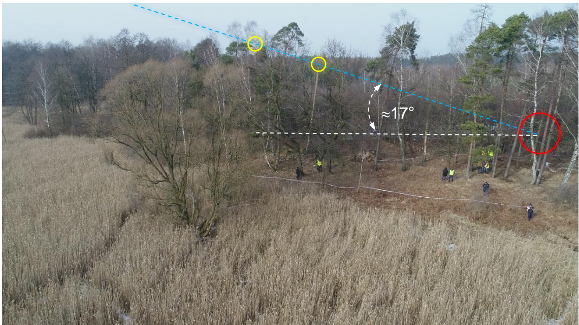
Fig. 19. Accident site – vertical plane through the helicopter flight path: the blue dotted line connecting two boughs with cut tops (yellow circles) shows the angle of descent (about 17°), the helicopter wreckage is marked with the red circle [source: PKBWL]
