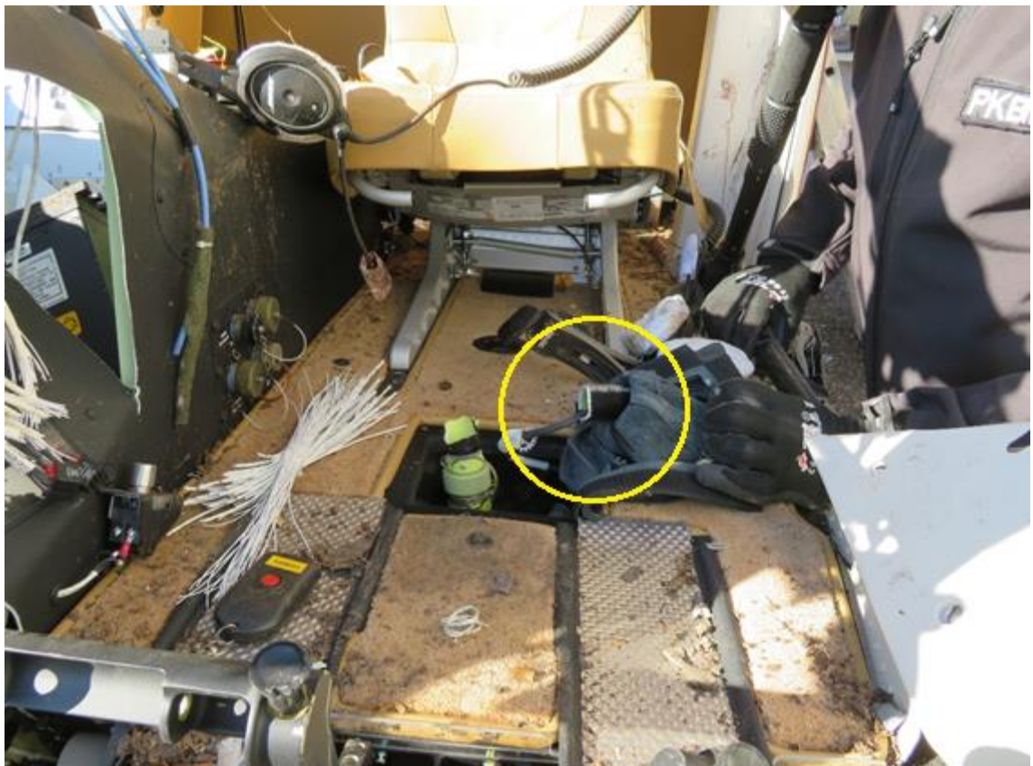
Fig. 27. The front passenger's seat: visible, broken control stick, marked with a yellow circle. [source: PKBWL]
