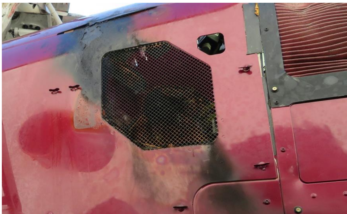
Fig. 21. Signs of fire found in the area of the left engine cowl [source: PKBWL]
