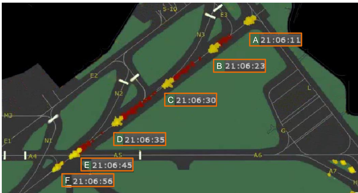
Fig. 2. FDB1830 aborted take-off: A – take-off run initiation, B – instruction to abort take-off, C – acknowledgement of the instruction, D and E – speed reduction, F - stop [source: PANSА, PKBWL]
