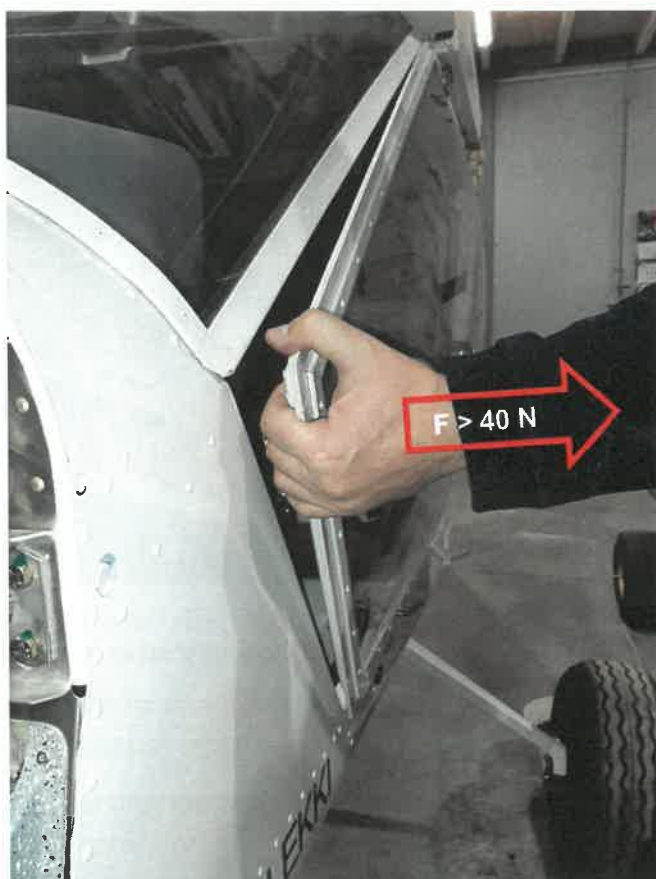
Fig. 8. The force above 40N applied to the door in its front area and a visible gap between the door and fuselage frame
