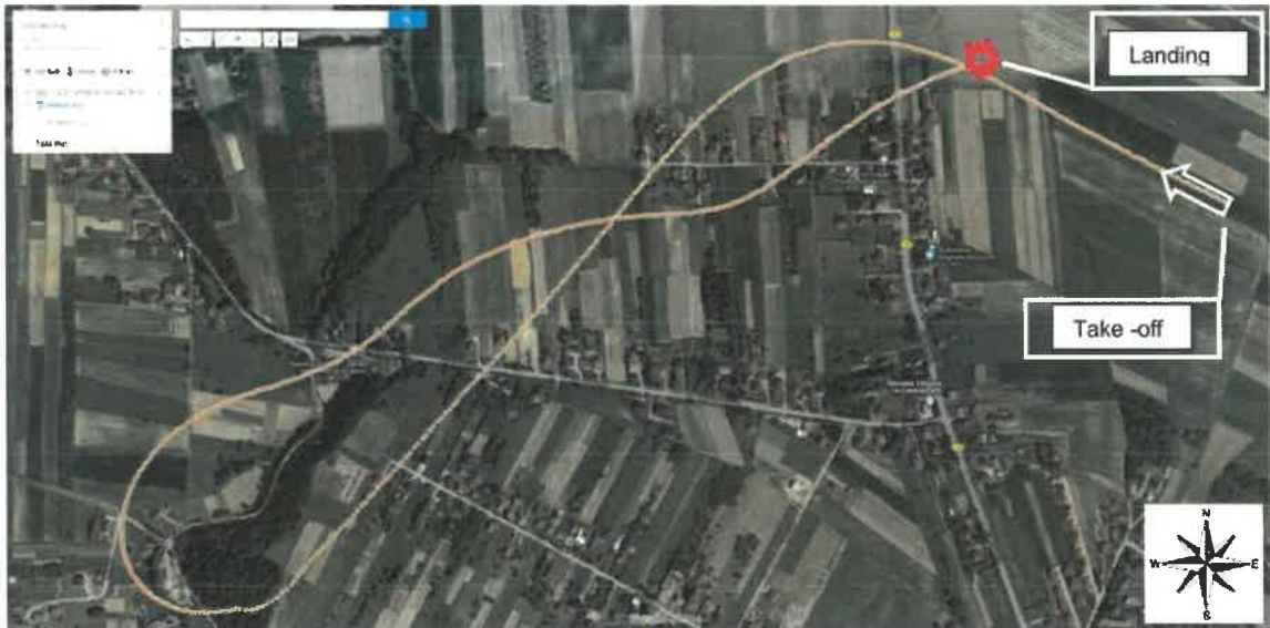
Fig. 1. Place of take-off and unintended landing. Flight trajectory established based on coordinates recorded by the flight computer installed on SP-SENO a/c [source: GoogleMyMaps]
