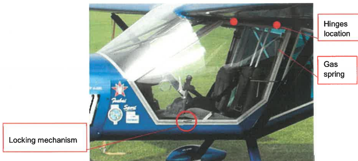
Fig. 7. Location of hinges and the locking mechanism on the door
