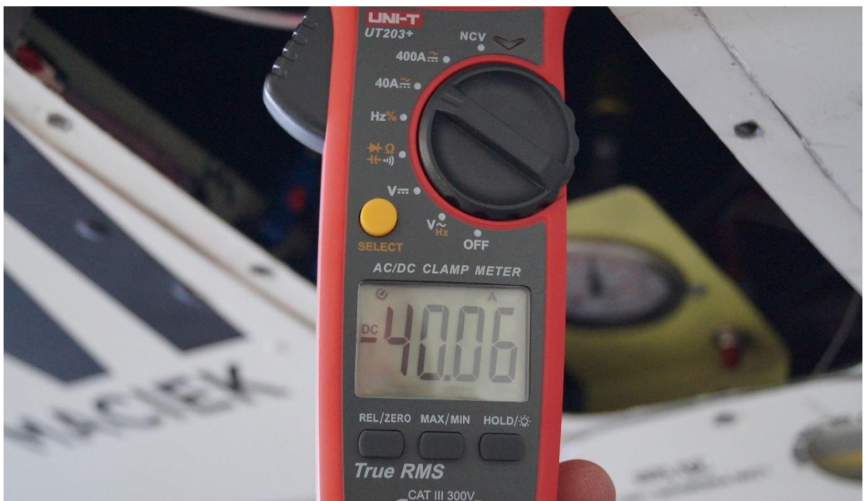
Fig. 5. Measurement of the current flowing through the landing gear extension and retraction system electric relays, photographed during the test
