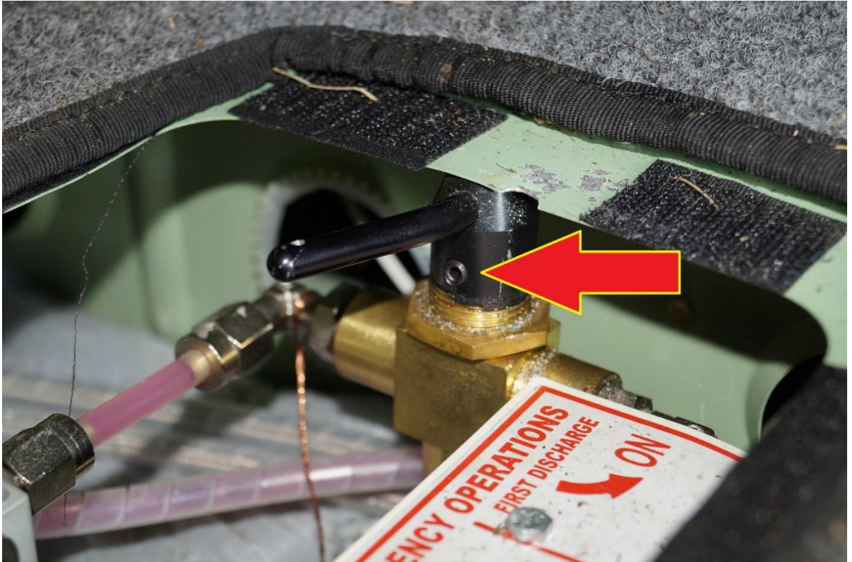
Fig. 11. Connection of the lever with the right-hand valve of the alternate landing gear extension system. The arrow marks the grub screw that prevents the free rotation of the lever on the valve shaft
