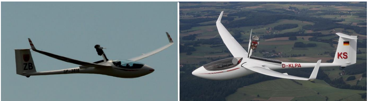
Figure 12. Position of the mast in flight: left – in the sailplane involved in the accident, right – the correct position [source: Dariusz Deptula, Internet]
