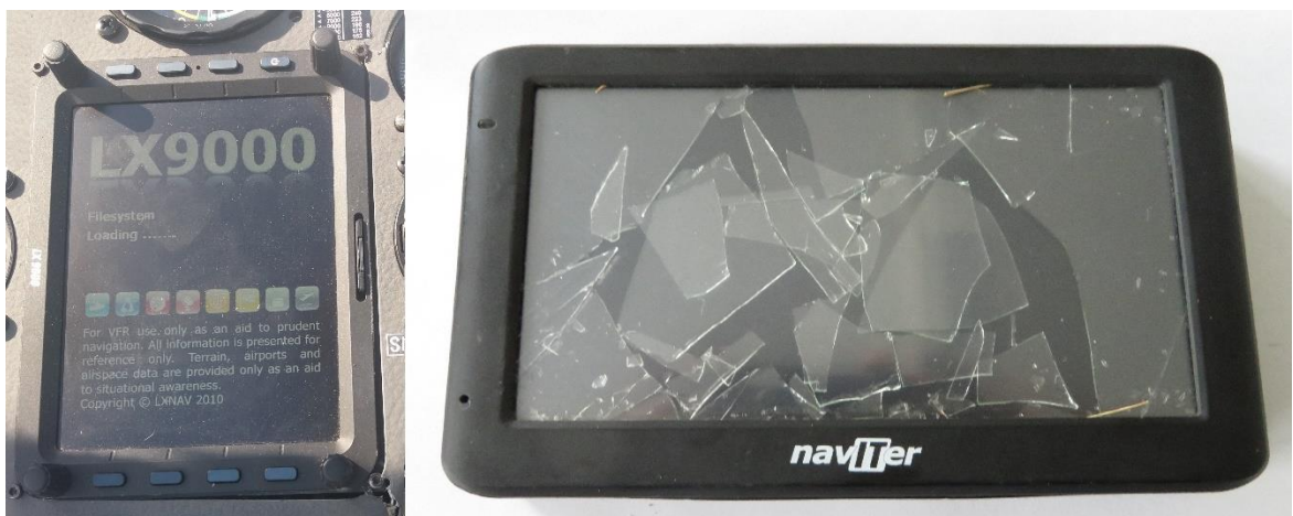
Figure 6. Flight recorders. On the right is the damaged Naviter Oudie IGC [source: PKBWL]
