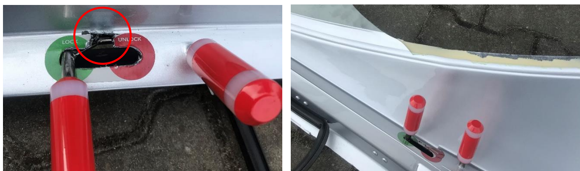
Fig. 9 Handles and sliders locking the canopy: rear (on the left) and front (on the right) [source: SCAA]
