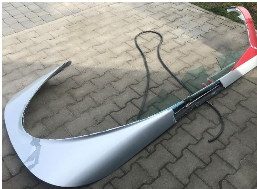
Fig. 3 Piece of canopy frame found [source: SCAA]
