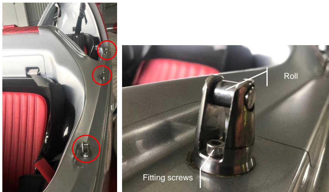
Fig. 6 Fittings for pawls on the portside [source: SCAA]
