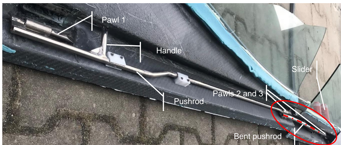
Fig. 7 Pawls on the common pushrod [source: SCAA]
