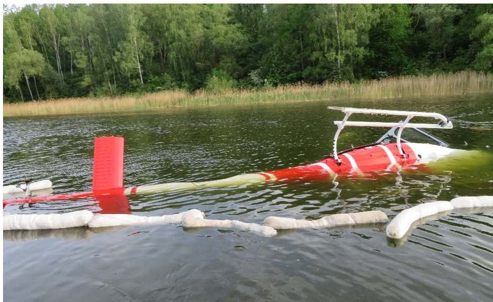
Fig. 1 Accident site – Eurocopter AS350B3e helicopter submerged in the lake and white absorbent sleeves deployed to collect contamination.
