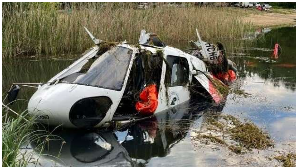
Fig. 2 The helicopter wreckage while being pulled onto the shore of the lake. Note the missing rotor and detached main gearbox.
