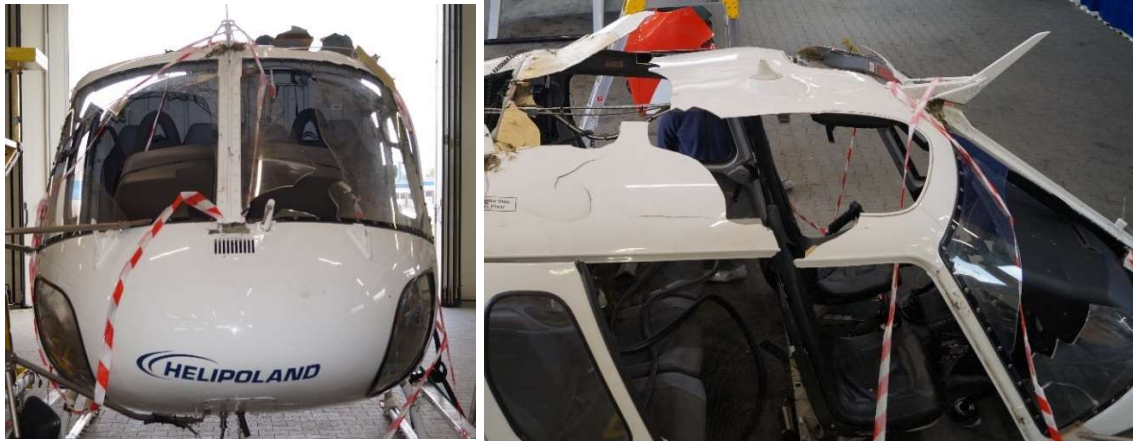
Fig. 9 External damage to the cockpit: breaches in the roof and large glazing fragments missing. The right-hand door is missing because it was released during evacuation.
