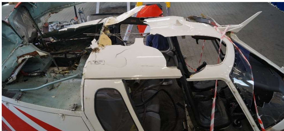
Fig. 3 The damaged fuselage of the helicopter and the place of the missing main gearbox.
