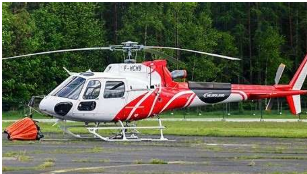
Fig. 4 Eurocopter AS350B3e helicopter and a bambi bucket designed to carry water [source: airplane-pictures.net]
