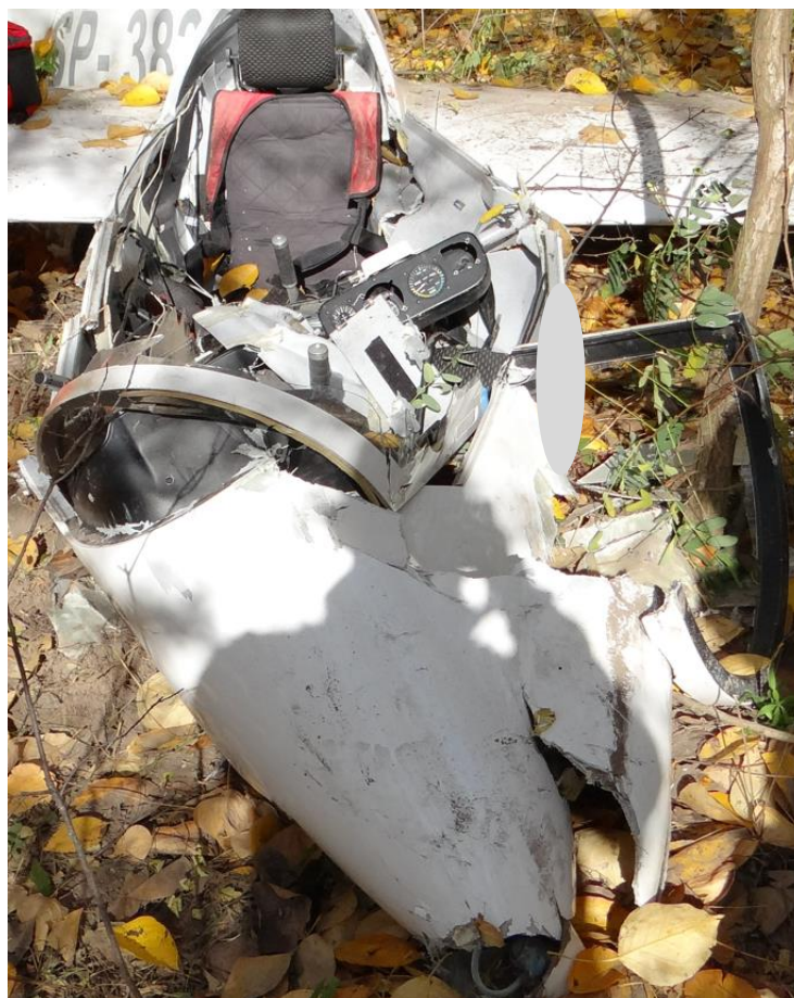
Fig. 3. Damage to the cockpit [source: SCAAI]
