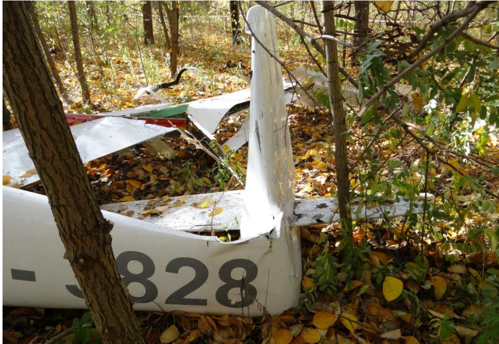
Fig. 5. Crushed and broken tail and torn right wing [source: SCAA]
