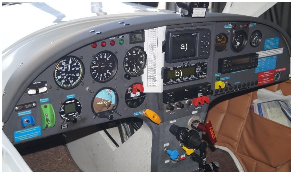
Fig. 12. Towing plane instrument panel: (a) GPS Garmin 296, (b) FlyDat to monitor Rotax engine [source: SCAAI]
