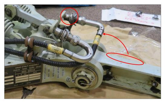
Fig. 4. Drag Strut Assembly - the red circle shows the place of the Proximity Sensor (NGLK2) collision with its target. The red ellipse shows the loss of the paint coating on the Lower Drag Strut and the arrow shows the direction of movement [source: SCAAI].
