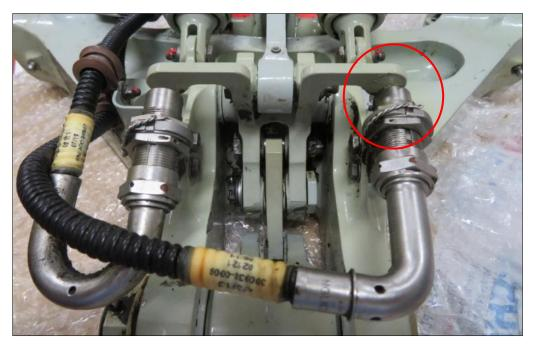
Fig. 5. Drag Strut Assembly – the red circle indicates the collision of the Proximity Sensor (NGLK2) with its target [source: SCAAI].
