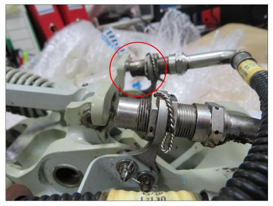
Fig. 6. Drag Strut Assembly – the red circle indicates the collision of the Proximity Sensor (NGLK2) with its target [source: SCAAI].
