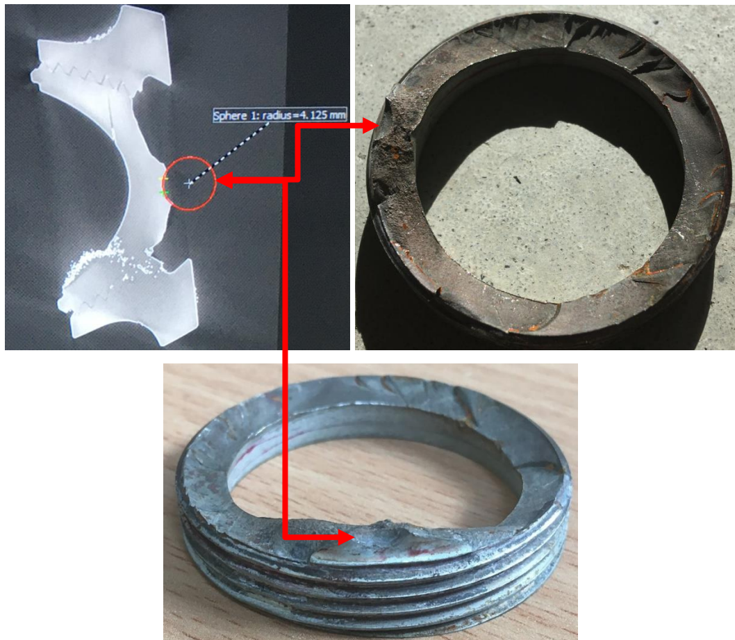
Fig. 15. Spherical breakage area [source: Warsaw University of Technology]
