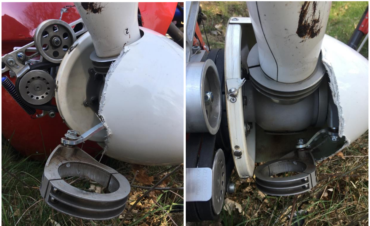
Fig. 3. Damaged propeller hub of the gyrocopter
