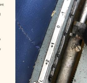
Seven detents for the flap control lever.
