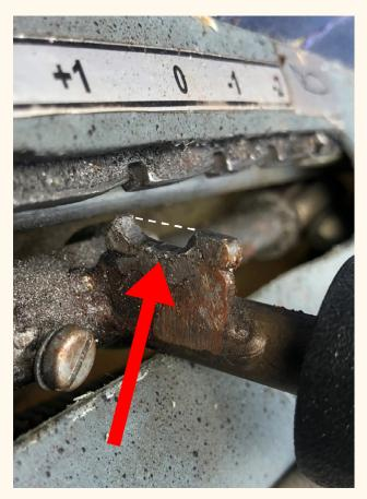
The pawl, with a notch in it, which is part of the flap control lever.
