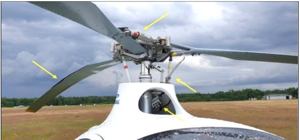
Fig. 4. SP-NCA helicopter damage – main rotor head [source: ACSL LAW]
