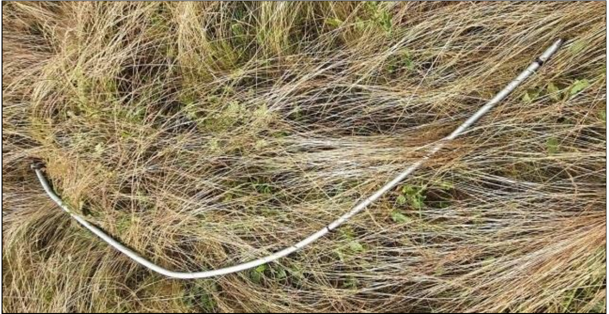
Fig. 8. Middle part of the fenestron drive shaft torn out from SP-NCA helicopter tail boom [source: ACSL LAW]
