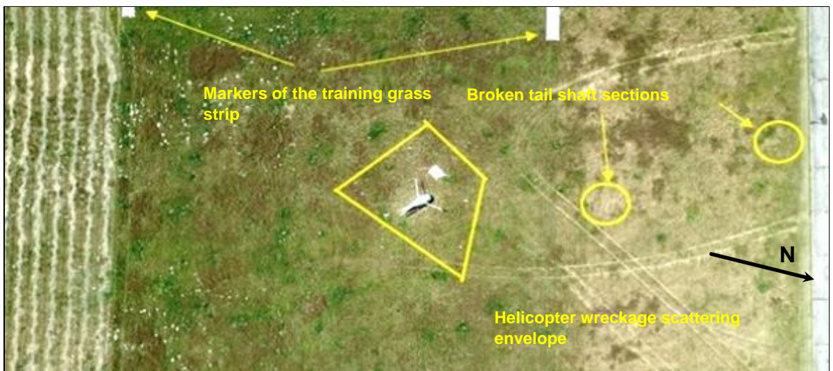
Fig. 12. Helicopter view at the occurrence site – scattering of wreckage [source: ACSL LAW, background: Google Earth]
