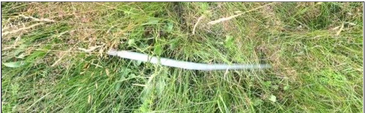
Fig. 9. End part of the fenestron drive shaft [source: ACSL LAW]
