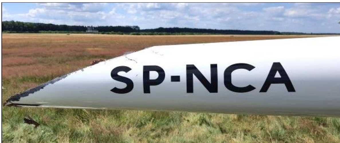
Fig. 6. Sheared tail boom [source: ACSL LAW]
