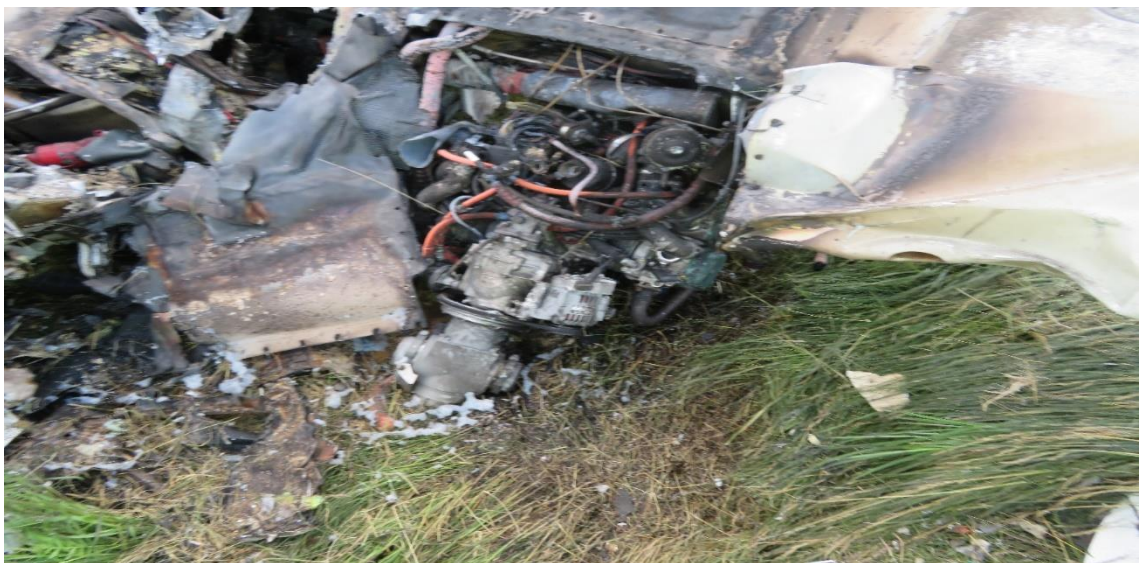
Fig. 6. Damaged powerplant unit no 1 [source: PKBWL]
