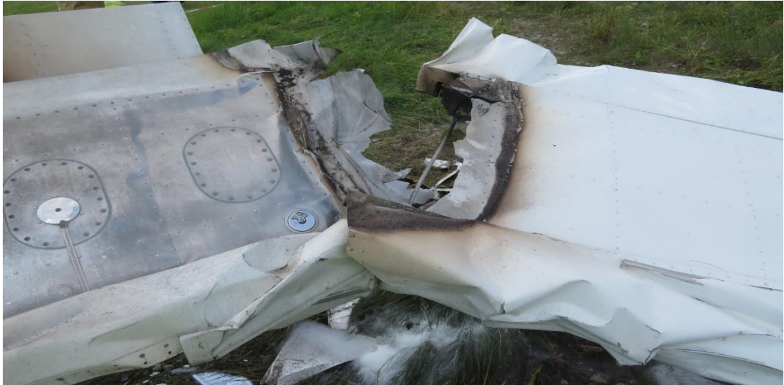
Fig. 5. Torn and deformed part of the left wing structure [source: PKBWL]
