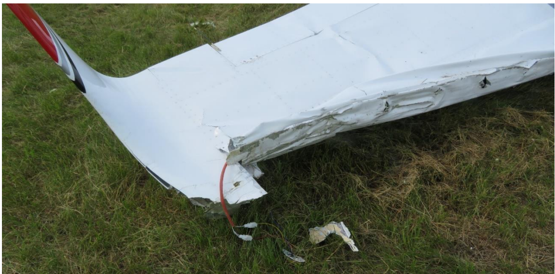
Fig. 4. Flat damage on the wing leading edge [source: PKBWL]
