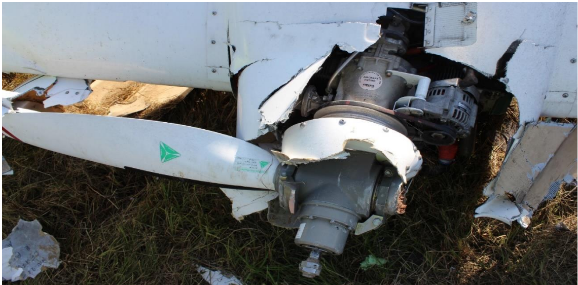
Fig. 7. Damaged engine no 2 [source: PKBWL].
