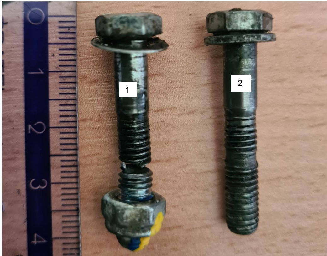
Fig. 1. Broken (1) and damaged (2) bolt of the stabilator suspension [source: PKBWL]
