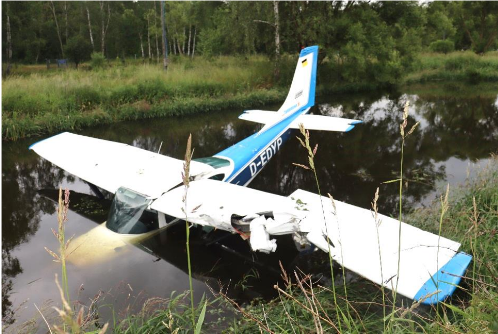
Fig. 1 The Cessna C-182L Skylane after the collision with the tree, embankment and water surface of the reservoir [source: the Police]
