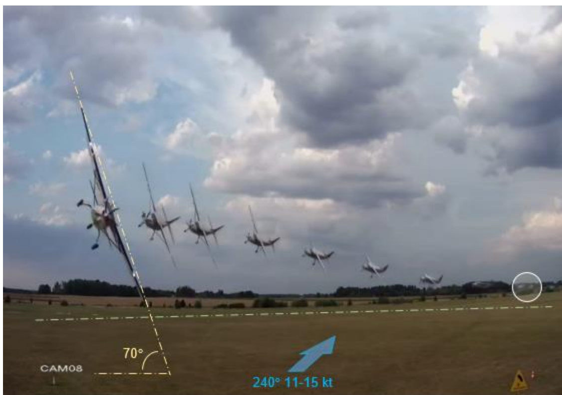
Fig. 1. Cessna 208B SP-WAW, in the flight after TAG, where: white circle – flight instructor takes control, yellow dashed line – bank angle, green dashed line – RWY centre line, blue arrow – approximate wind direction.
