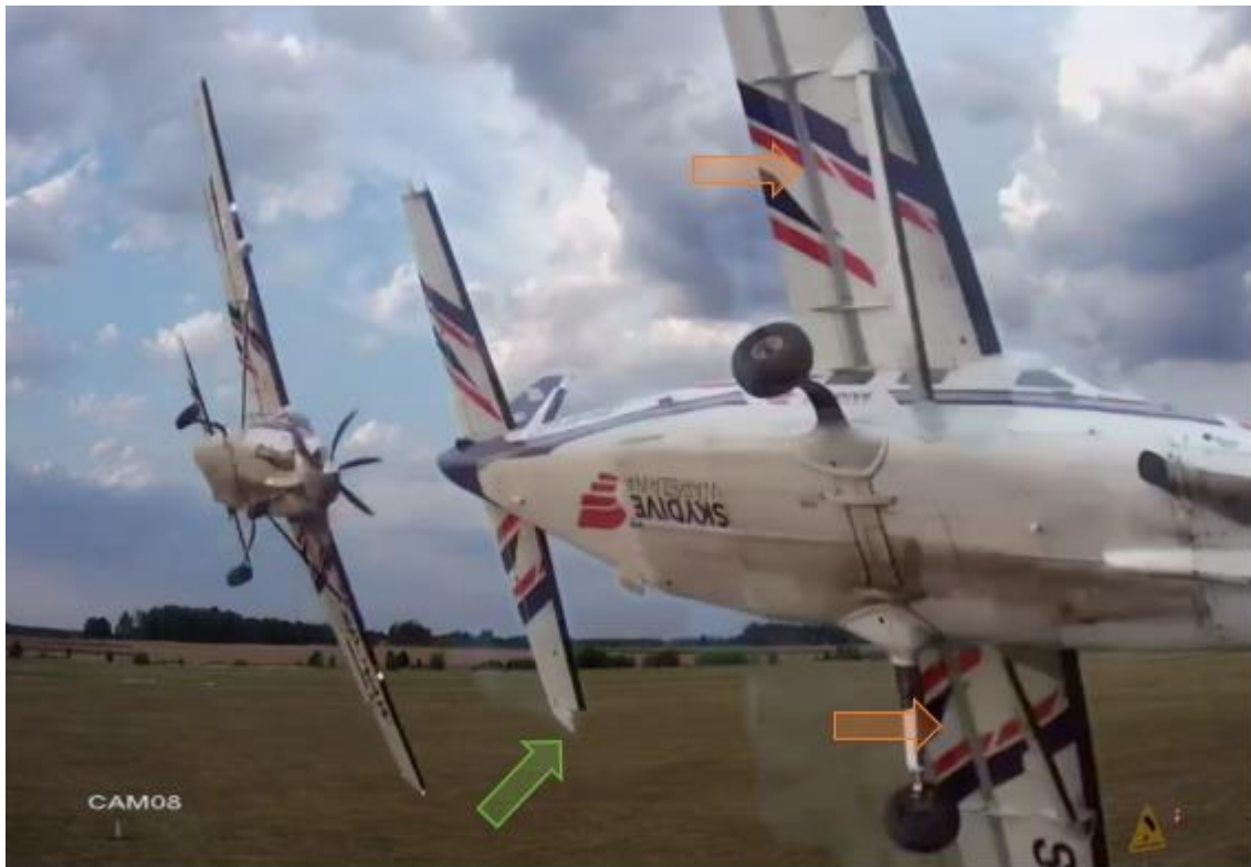
Fig. 2. Cessna 208B SP-WAW (next time-lapse photos - Fig. 1 continued), where: the right photo shows the moment of the left wing contact with the surface of the airfield, orange arrows show symmetrically extended wing flaps and green arrow shows the elevator deflected up.
