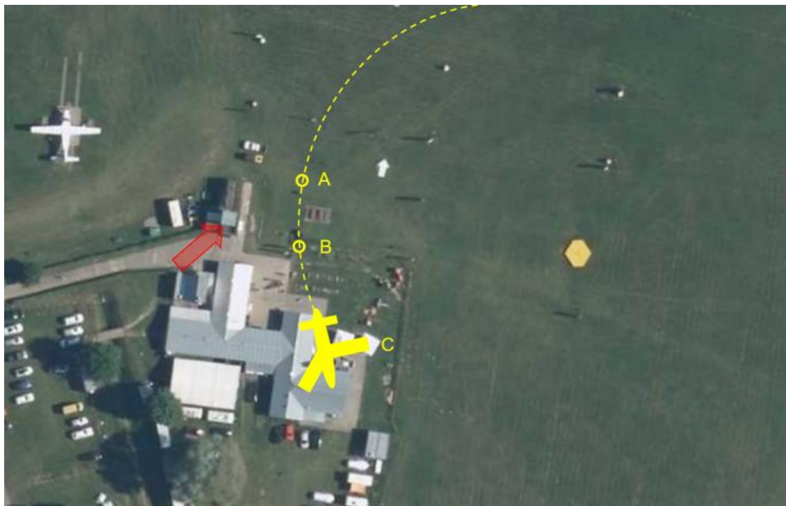
Fig. 7. Accident site. The following elements are marked in yellow: A – the place of the aircraft first contact with the ground (left wing tip); B – the place of the plane collision with the fence of the building; C – position of the wreckage. "Tower" of the airfield indicated by red arrow [source: https://mapy.geoportal.gov.pl ].
