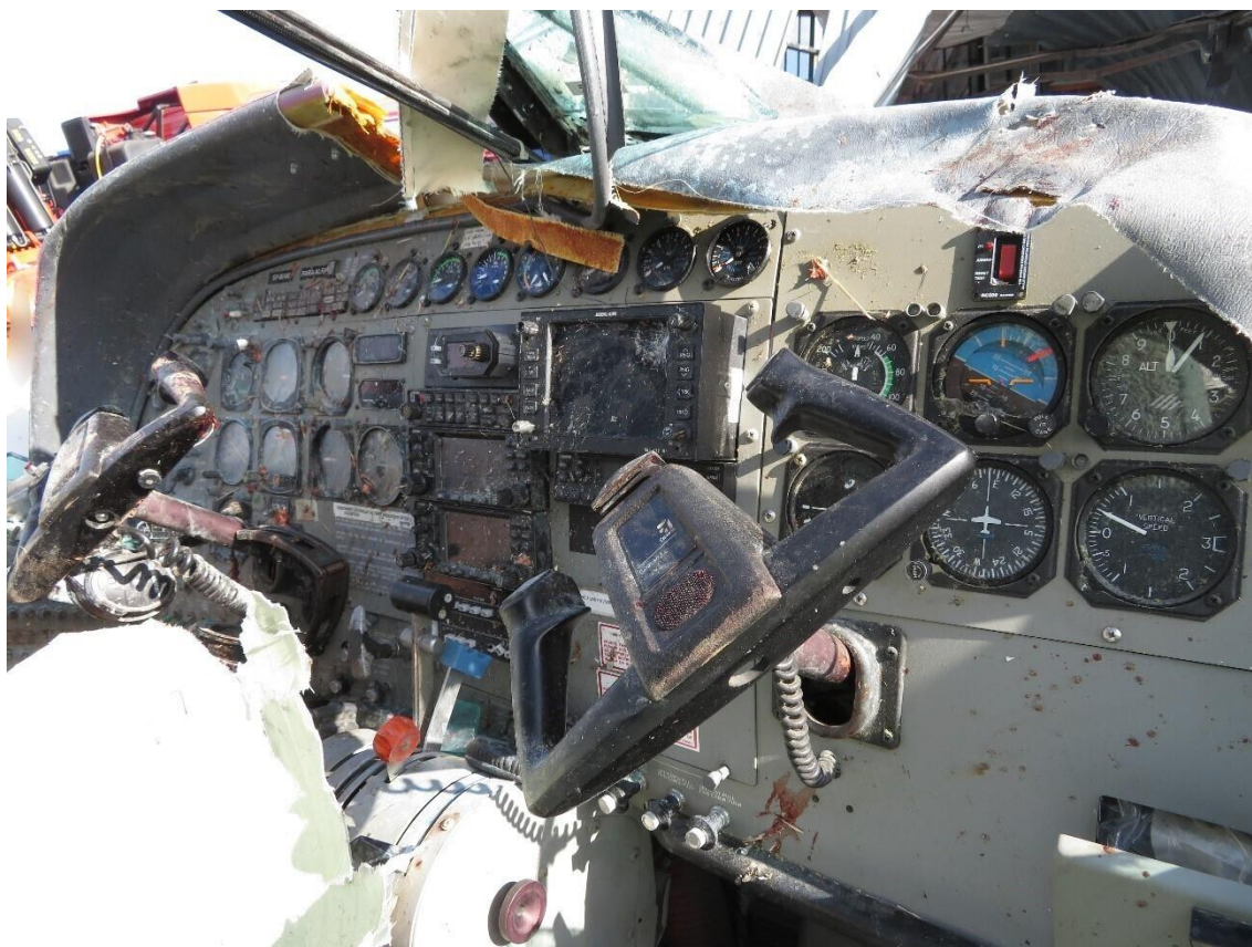
Fig. 9. Cockpit of Cessna 208B, SP-WAW after the accident. It is visible, that the right control wheel is clean in the places of hands location.
