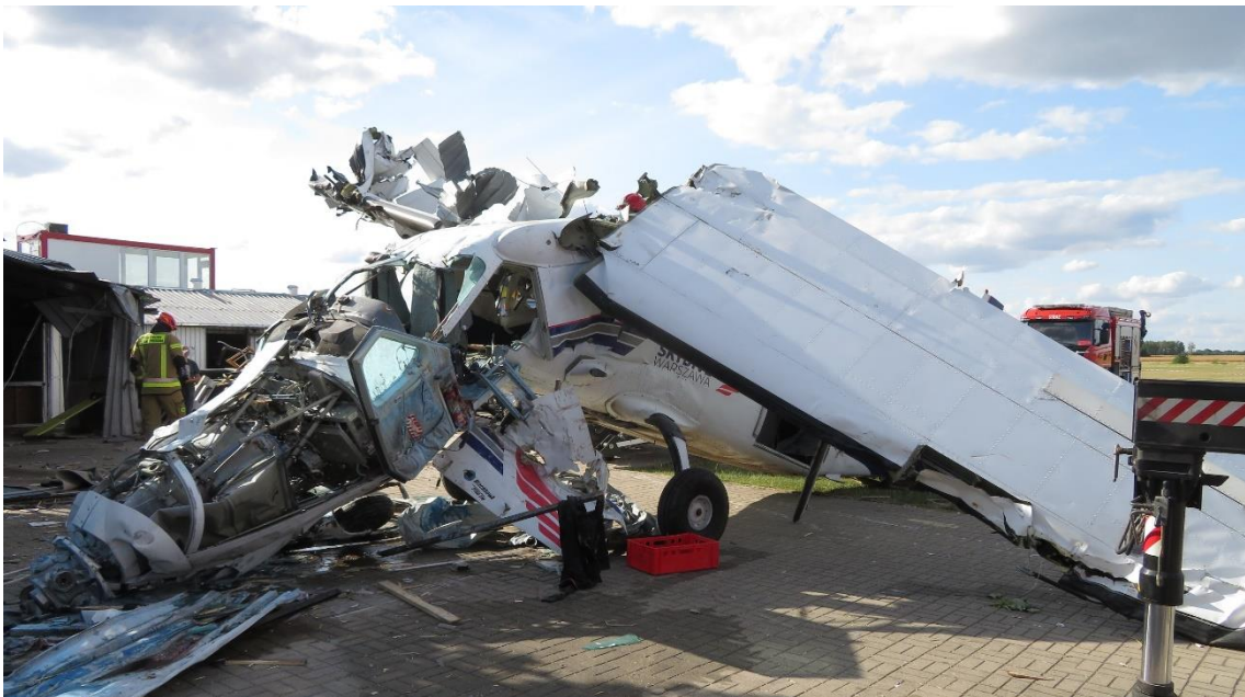
Fig. 3. Cessna 208B, SP-WAW – the wreckage after separation from the structure of the building.
