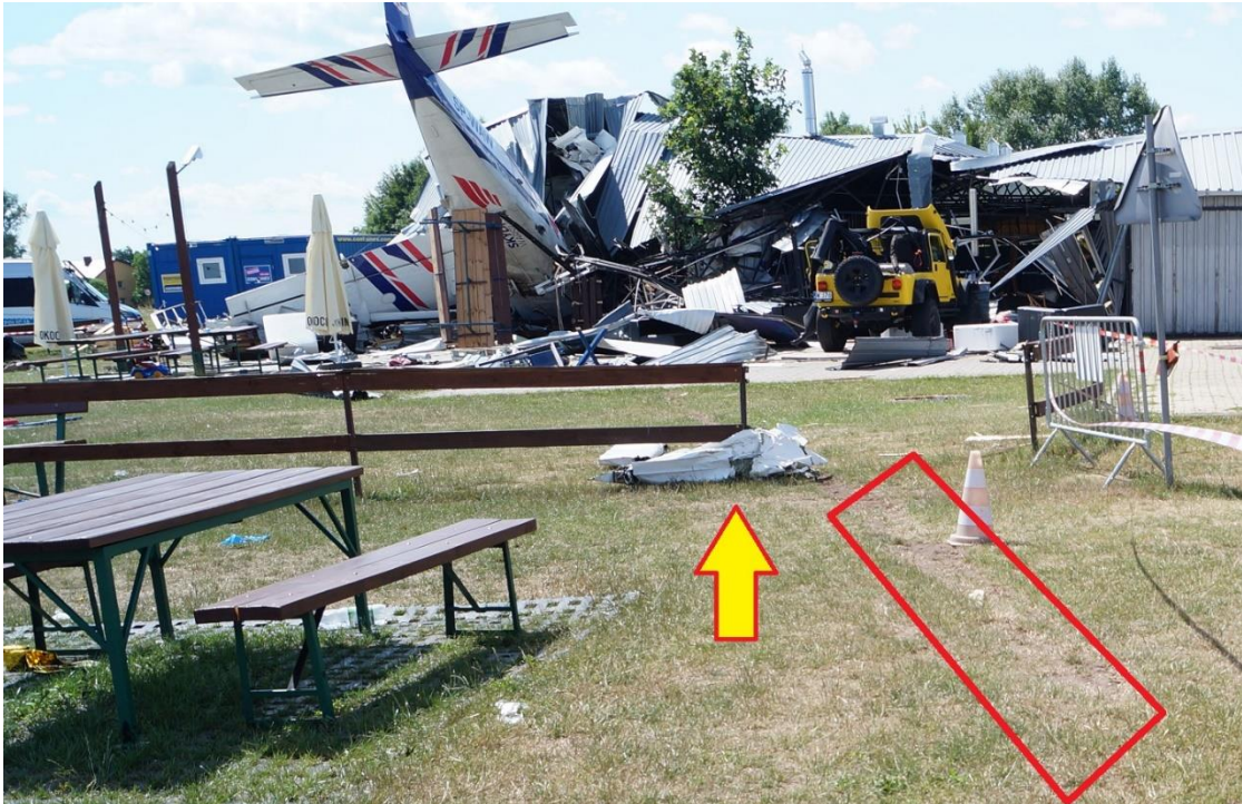
Fig. 8. Accident site. The red frame marks the trail of the left wing tip left on the grass in front of the building. The yellow arrow marks the tip of the left wing, which was torn off as a result of the collision of the wing with the building fence.
