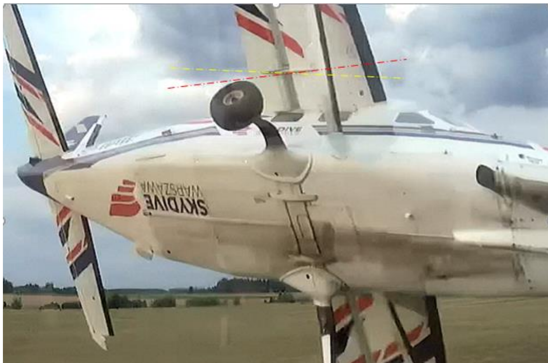
Fig. 15. Cessna 208B SP-WAW – enlargement of one of the frames from aerodrome camera, where: red line - extension of the edge of the flap track, yellow line - extension of the edge of the flap support assembly.
