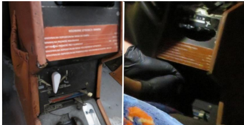
Figure 8. Location of the fuel valve lever after the occurrence. Attempt to change the location of the fuel valve lever.
