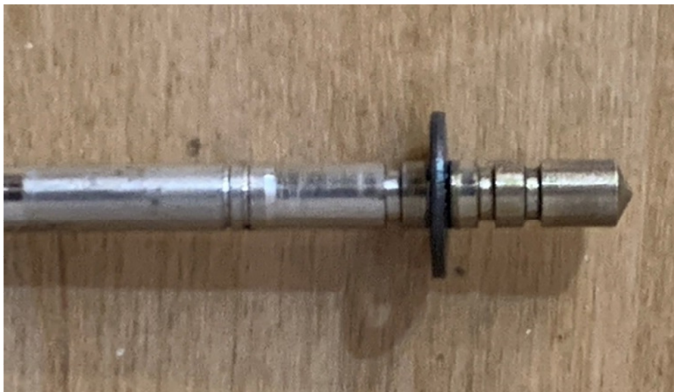
Fig. 18 The carburettor needle and its setting [source: PKBWL]
