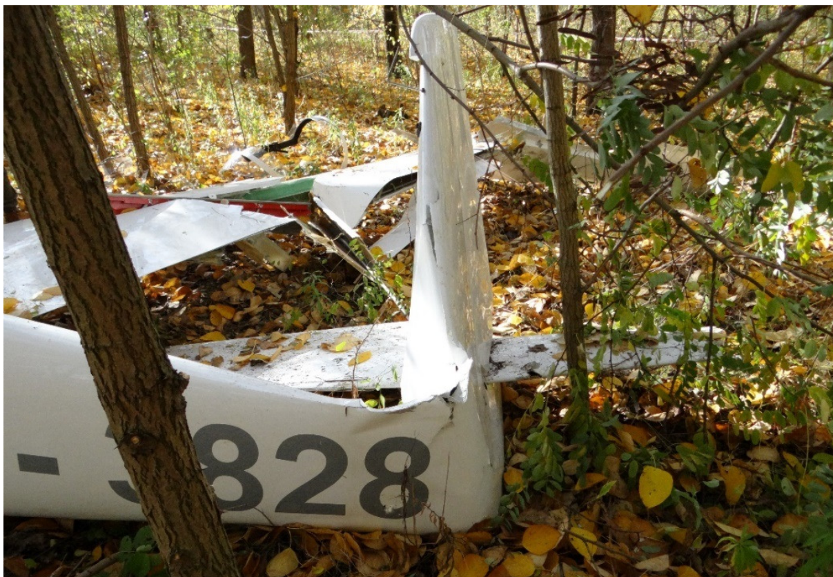
Fig. 3 The crushed and broken tail, and the torn right wing [source: PKBWL]
