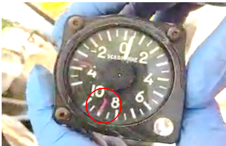
Fig. 13 The g-meter found in the wreckage – a frame from a video recording from the accident site [source: PKBWL]
