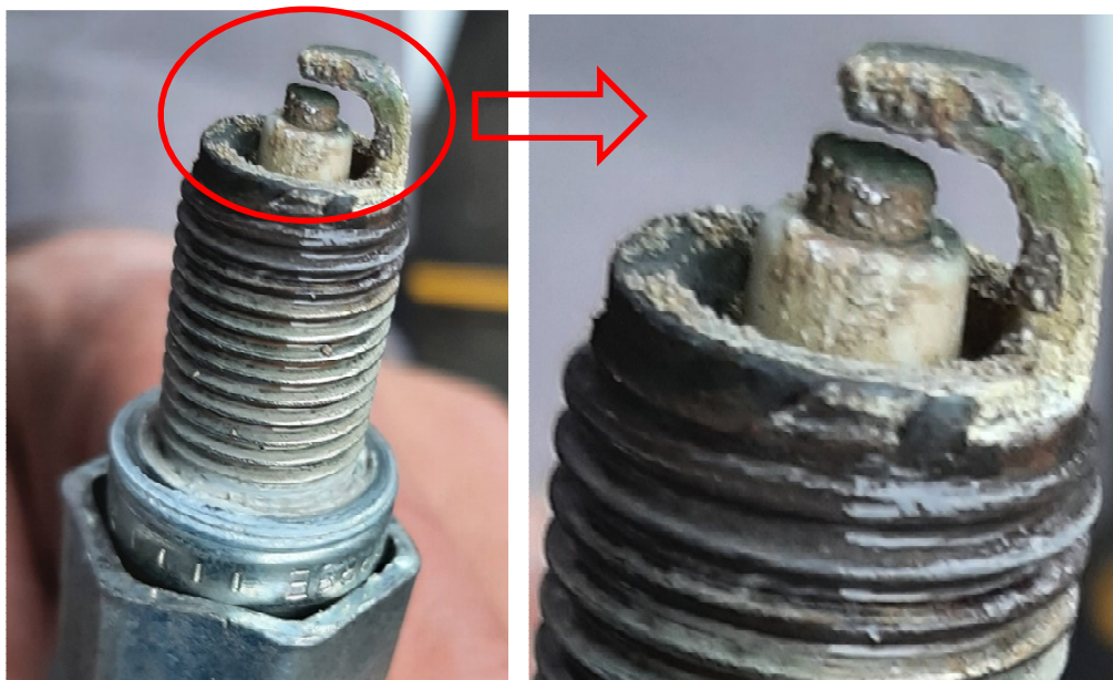
Fig. 14 Carbon deposit on the electrode of the spark plug of cylinder no. 1 [source: PKBWL]
