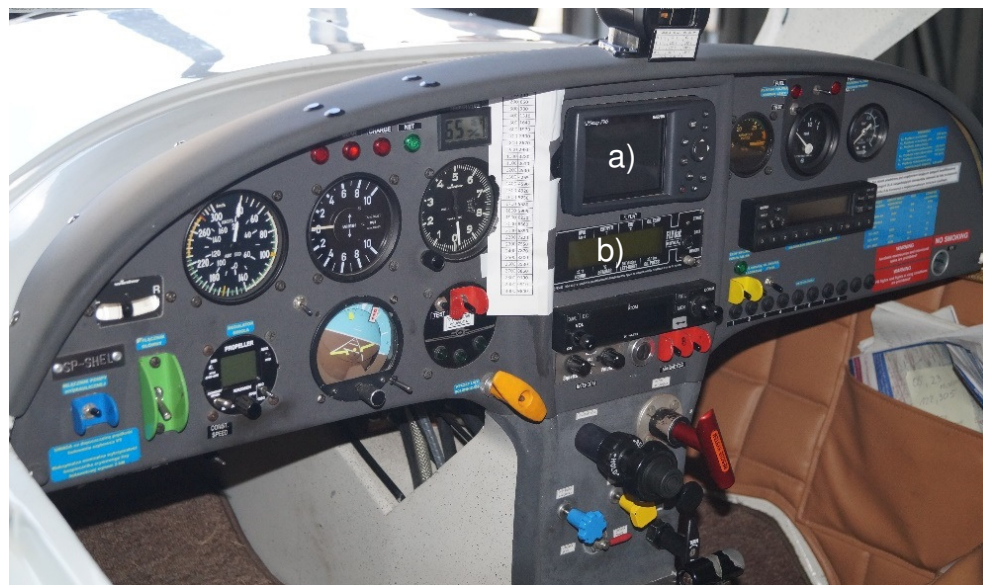
Fig. 11 The tow plane's instrument panel: (a) GPS Garmin 296, (b) FLYdat [source: PKBWL]
