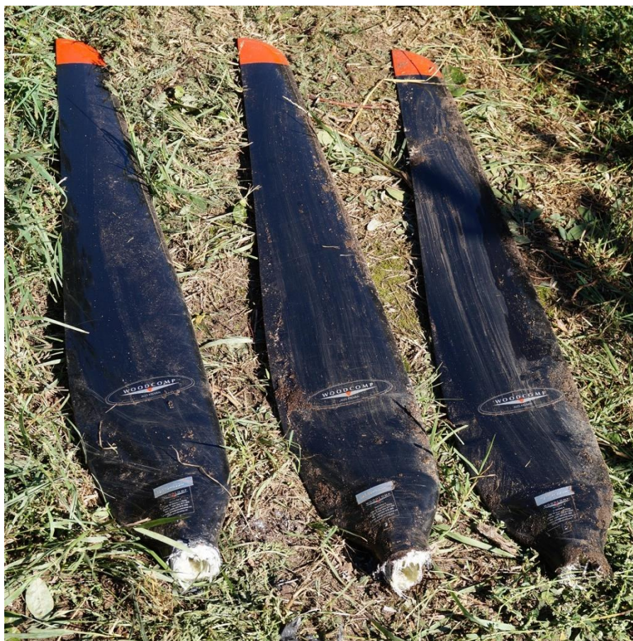
Figure 6. The propeller blades of the Storch CL OK-TUV 61 recovered from under the wreckage.
