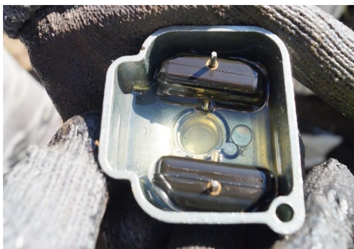
Figure 11. The carburettor float chamber of the Storch CL OK-TUV 61 with fuel found inside
