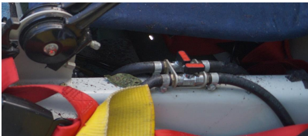
Figure 10. The fuel cocks of the Storch CL OK-TUV 61 after the accident. The closed right tank fuel cock and open left tank fuel cock can be seen.
