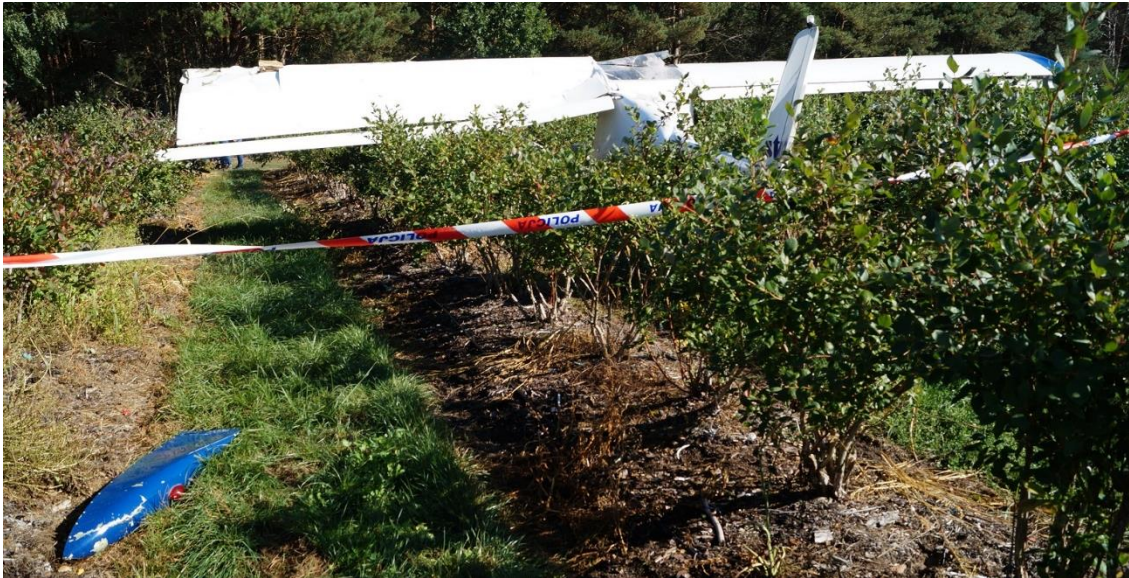
Figure 4. The Storch CL OK-TUV 61 at the accident scene. The left wing tip fairing can be seen in the bottom left corner of the picture
