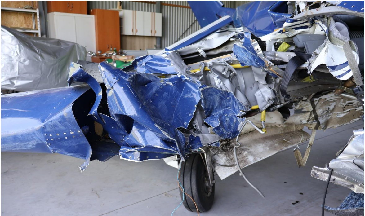
Figure 5. The damage caused by the aeroplane's impact on the edge of the roof.
