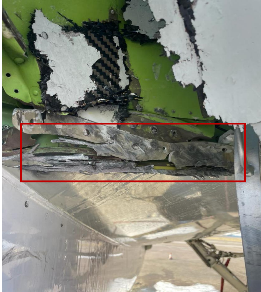
Figure 9. Damage to the connection between the lower wing skin and the front spar of the left wing between ribs 1 and 2. The marked area indicates the damage through which fuel leakage from the left-wing tank occurred.
