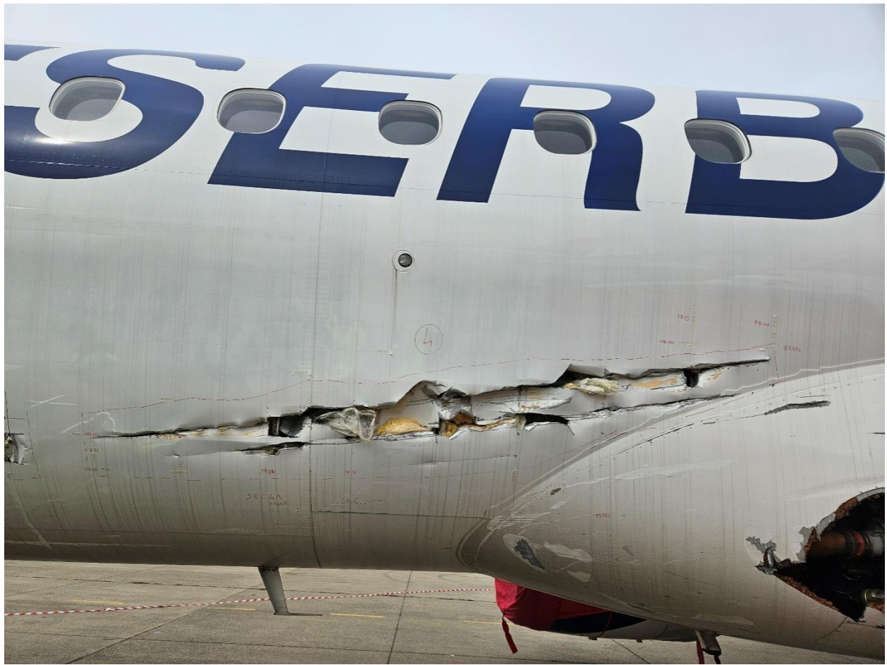
Figure 4. Zone 4 – Left side of the aircraft fuselage – continued contact between the fuselage and airfield equipment in the area between fuselage frames 32 and 40 and between stringers 17L and 22L
