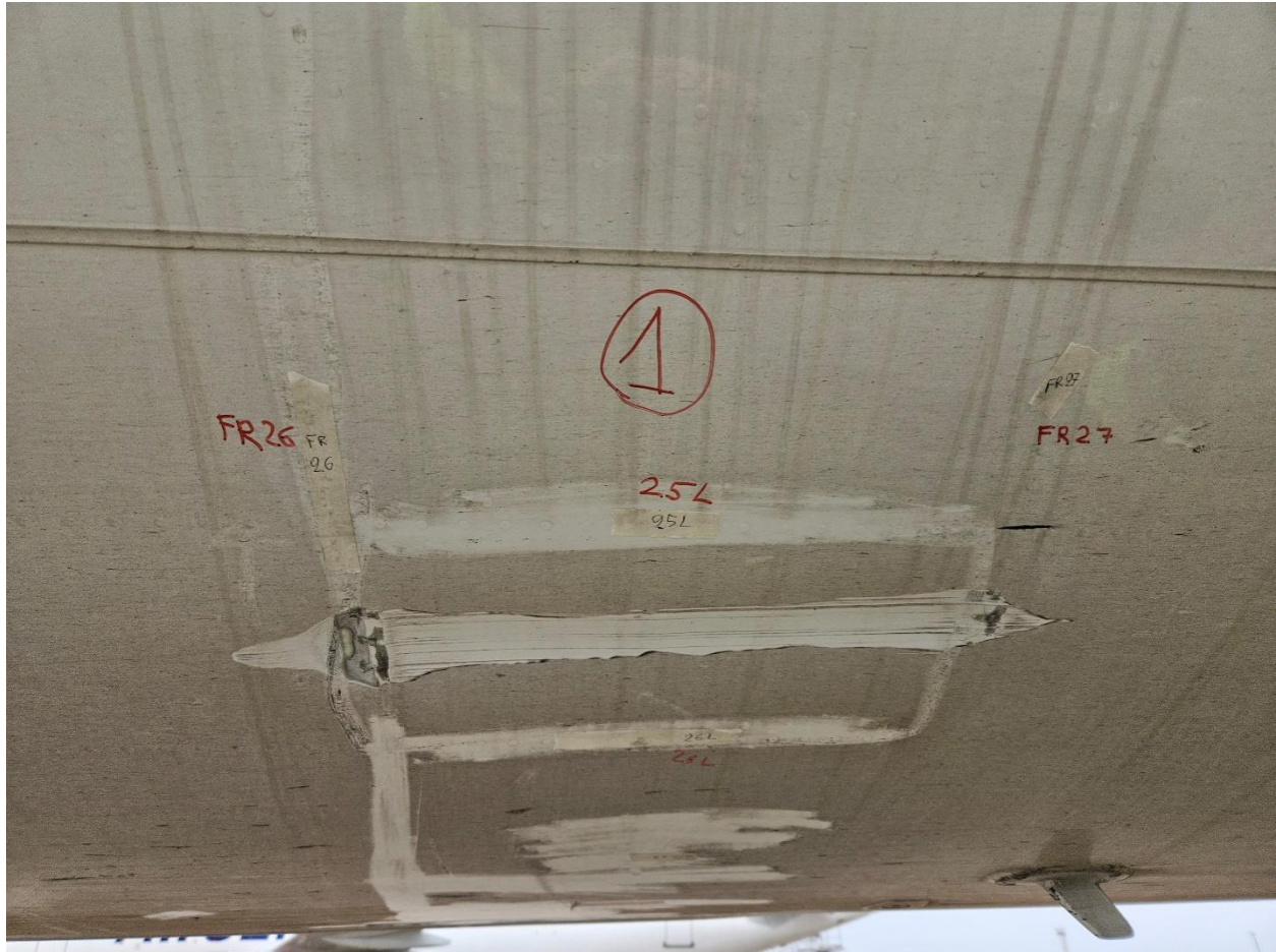
Figure 1. Zone 1 – Left side of the aircraft fuselage – initial contact between the fuselage and the airfield lighting in the area between fuselage frames 26 and 27 and along stringer 25L
