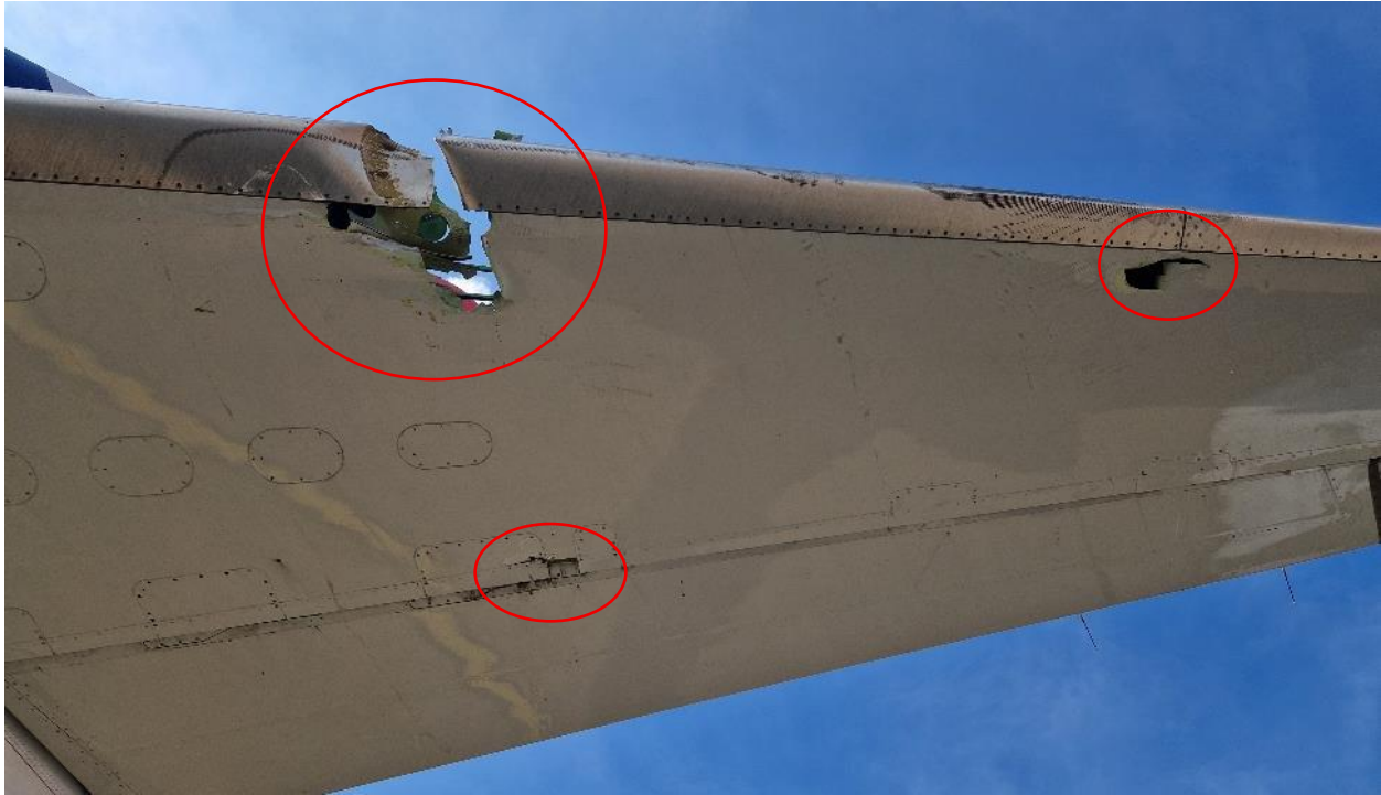
Figure 14. Damage to the leading edge between ribs 8 and 9 and to the lower skin of the left horizontal stabilizer
