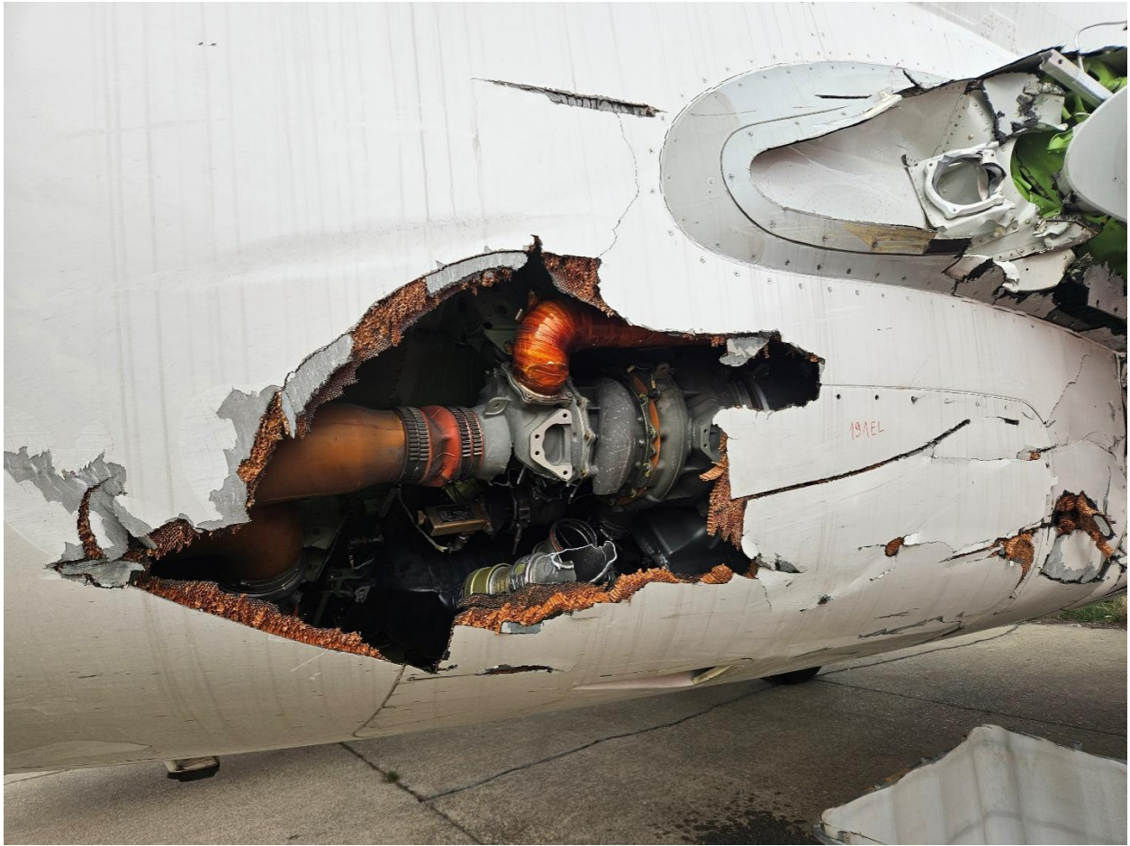
Figure 5. Damage to the composite panel in the lower wing-to-fuselage fairing area
