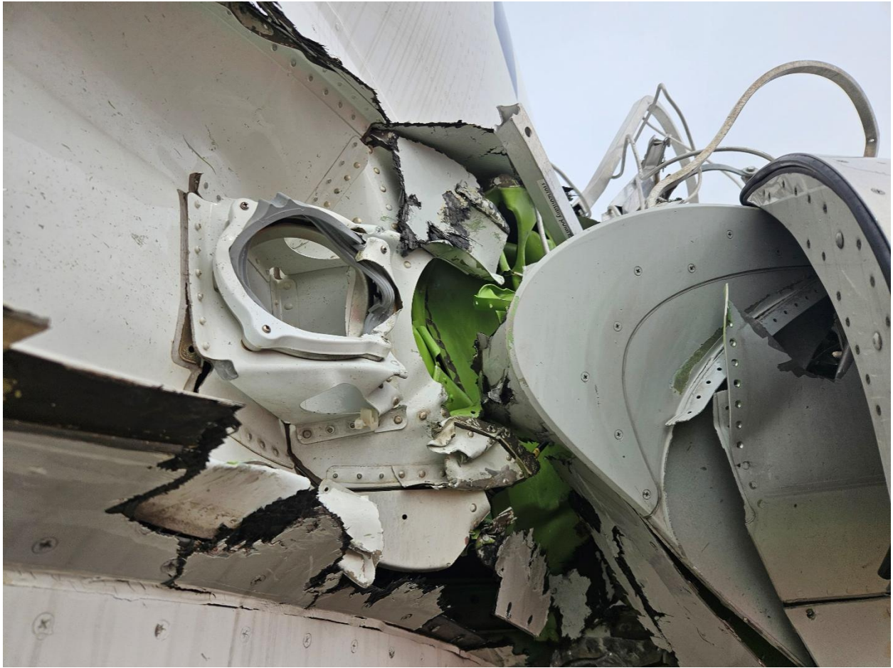
Figure 7. Impact area of the airport antenna mast at the root of the left wing
