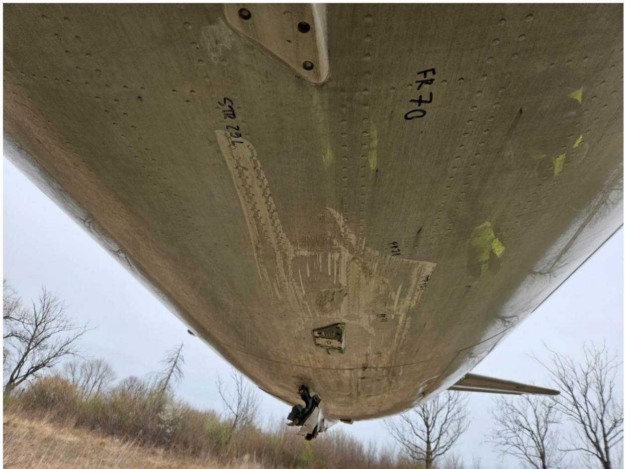
Figure 11. Damage to the lower fuselage skin in the area from fuselage frame 75 to frame 76 between stringers 27L and 29R
