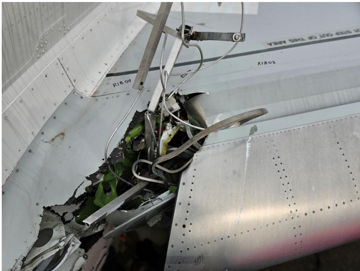
Figure 8. Parts of the airport antenna lodged in the wing root between ribs 1 and 3 of the left wing
