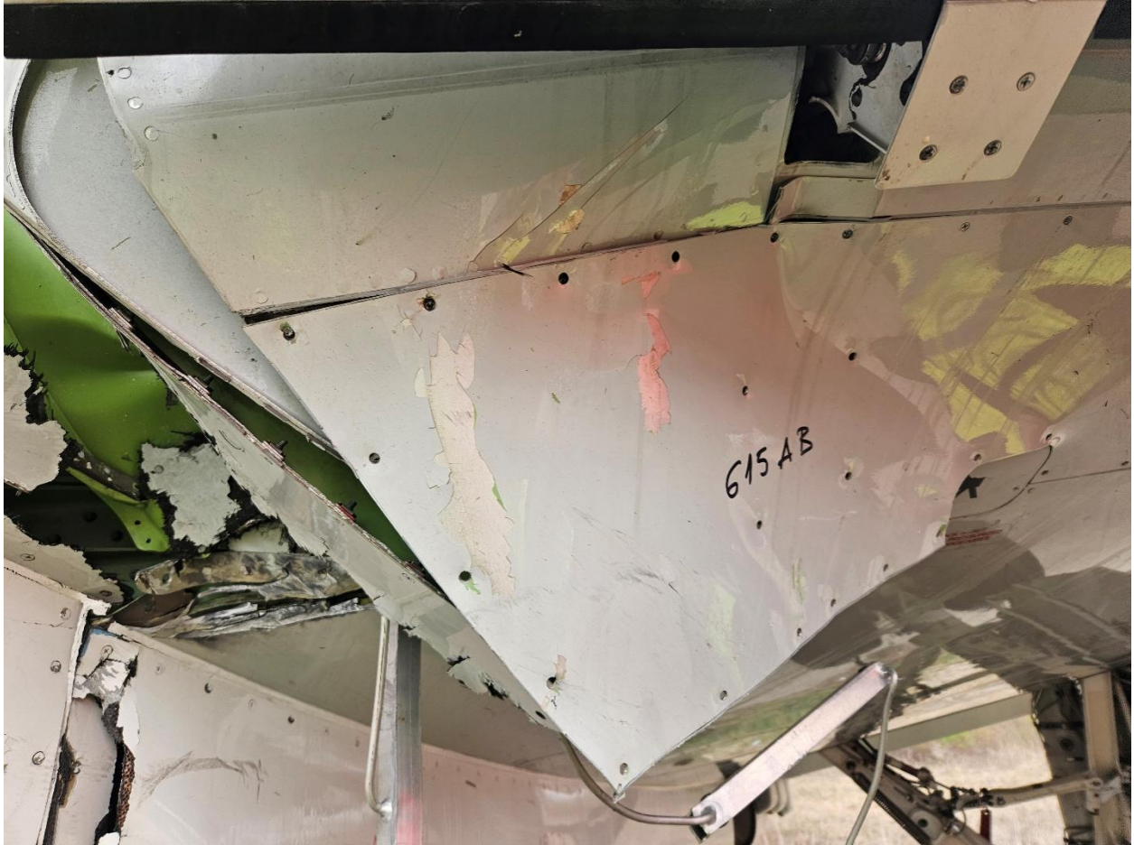
Figure 6. Damage to the lower skin of the left wing
