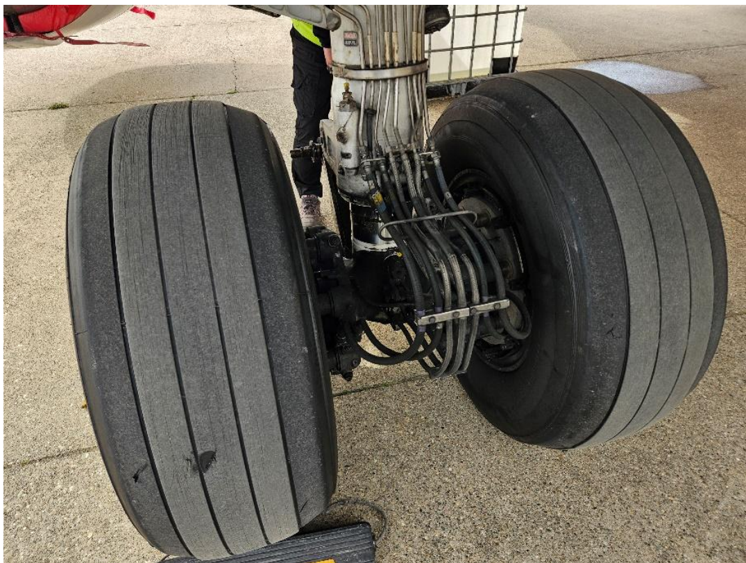
Figure 15. Left main landing gear wheels showing damage marks
