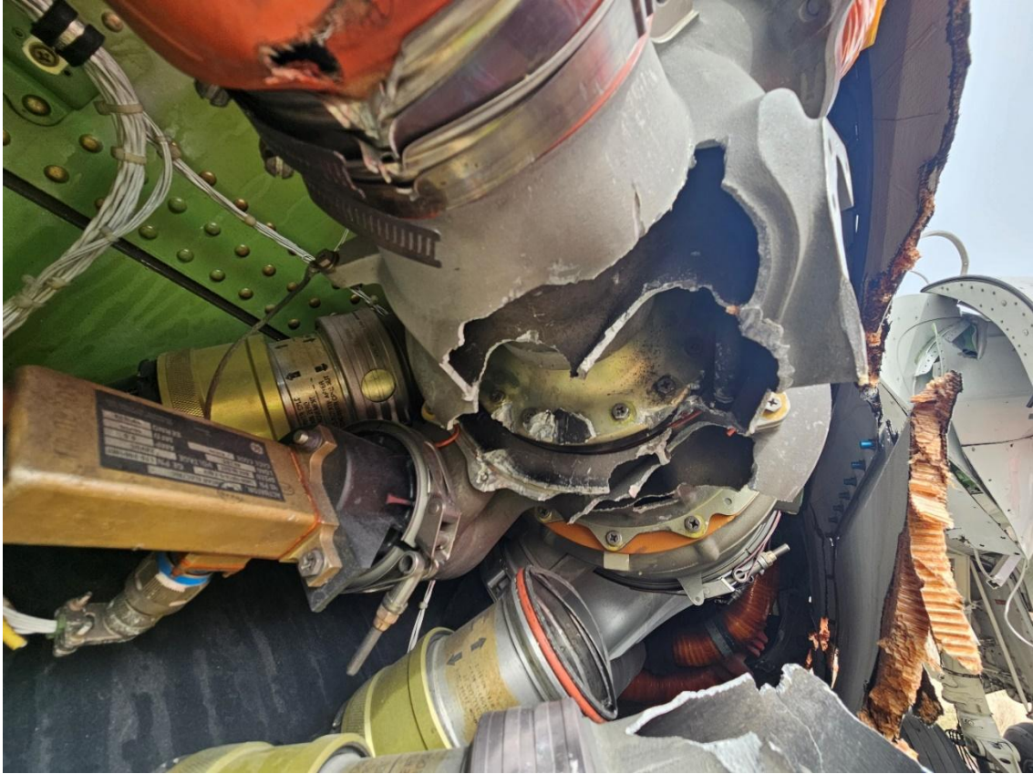
Figure 12. Damage to the left air conditioning system
