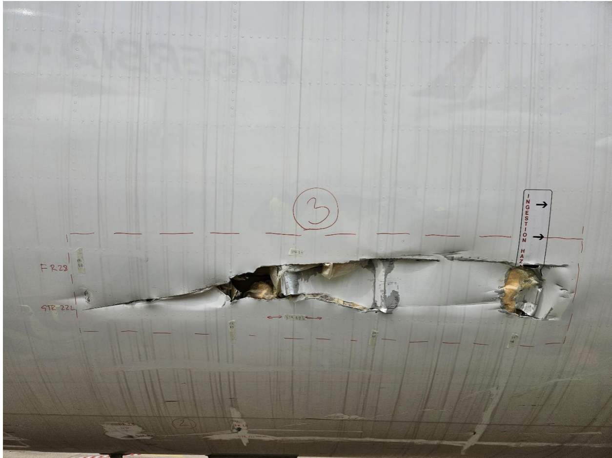
Figure 3. Zone 3 – Left side of the aircraft fuselage – continued contact between the fuselage and airfield equipment in the area between fuselage frames 28 and 31 and along stringer 22L
