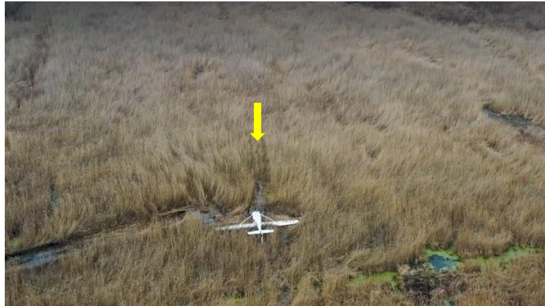
Fig. 2. The position of the aeroplane after overturn, with the touchdown point marked by a yellow arrow.
