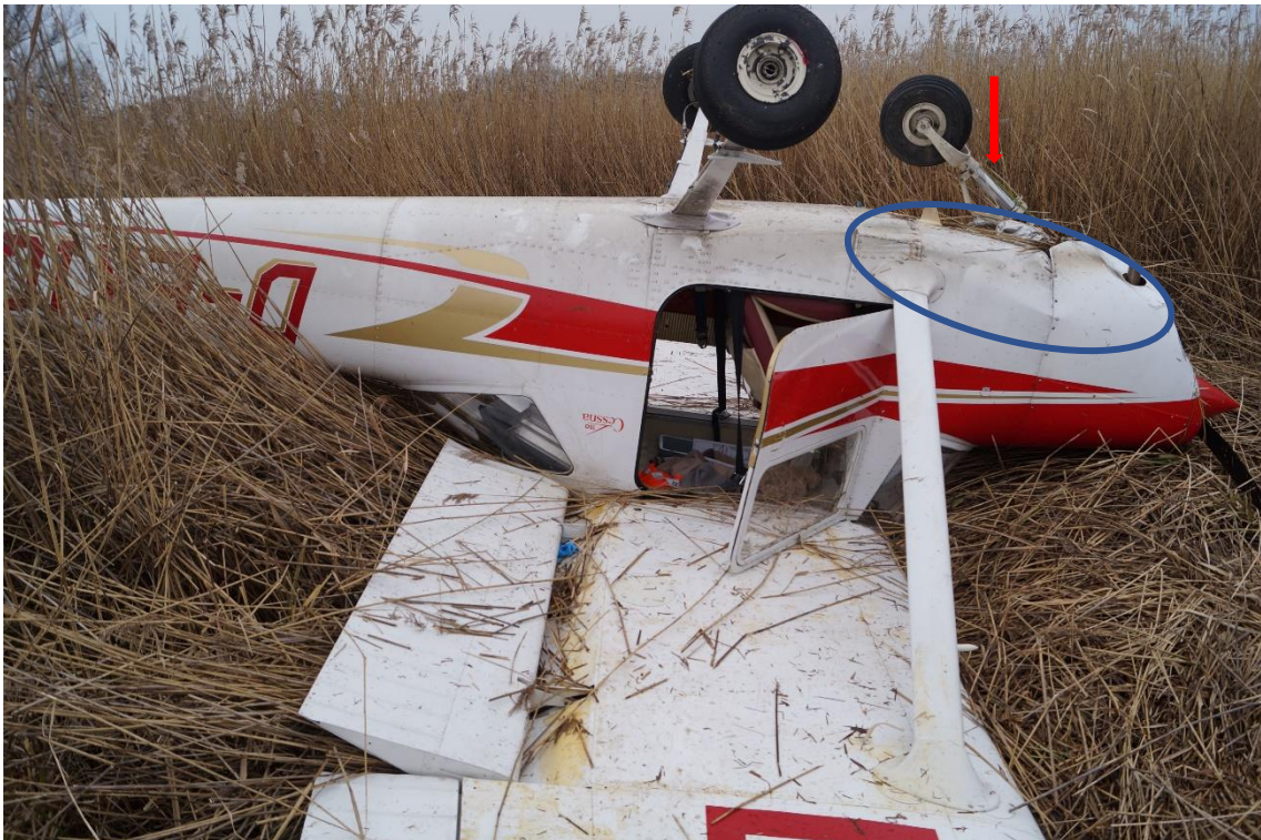
Fig. 5. A view of the damage to the nose section of the fuselage.
