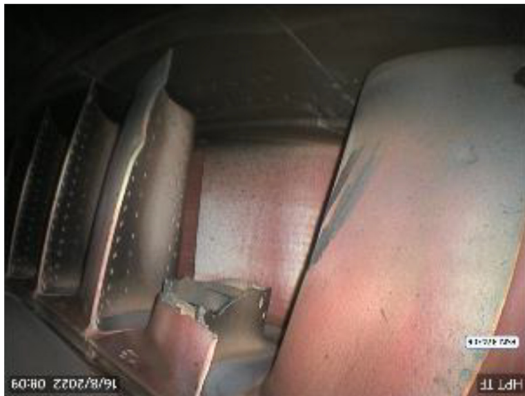
Fig. 2. HPT BSI results. Engine #2, HPT Blade #80 fracture at ~15% span, while multiple HPT blades and downstream hardware damaged due to impact from the liberated debris.
