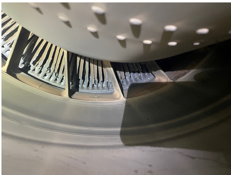
Fig. 3. Two pictures of stage 4 LPT blades of Engine #2 and downstream hardware damaged due to impact from the liberated debris.
