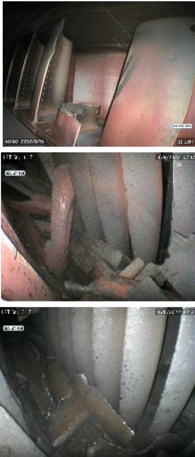
Fig. 17. Three pictures: HPT BSI results. Blade #80 fractured at ~15% span, while multiple LPT blades and downstream hardware were damaged due to impact from the liberated debris.
