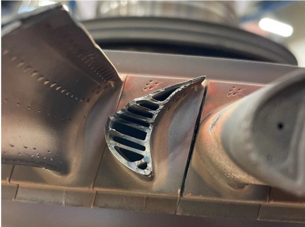
Fig. 18. Three pictures. Overview photos at HPT exposure. Blade #80. Multiple blades were damaged due to impact from the liberated airfoil debris.
