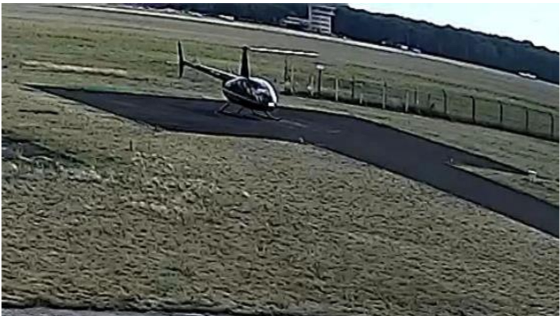
Figure 6. The initial attempt to take off, linear movement of approximately 1 m to the right with a simultaneous rotation of approximately 30° to the left with a forward tilt [source: CCTV footage].
