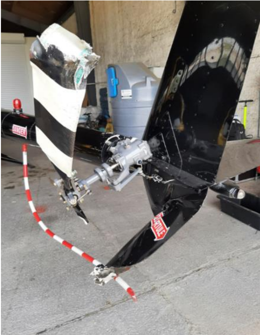
Figure 13. Broken tail skid, damaged lower vertical stabiliser and broken tail rotor bracket.
