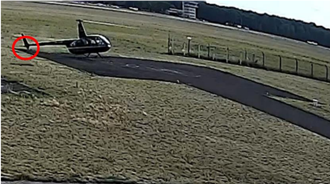
Figure 11. Just before the leftward rotation stops, hitting the helipad for the third time, destroying the tail rotor (marked with a red circle) [source: CCTV footage].
