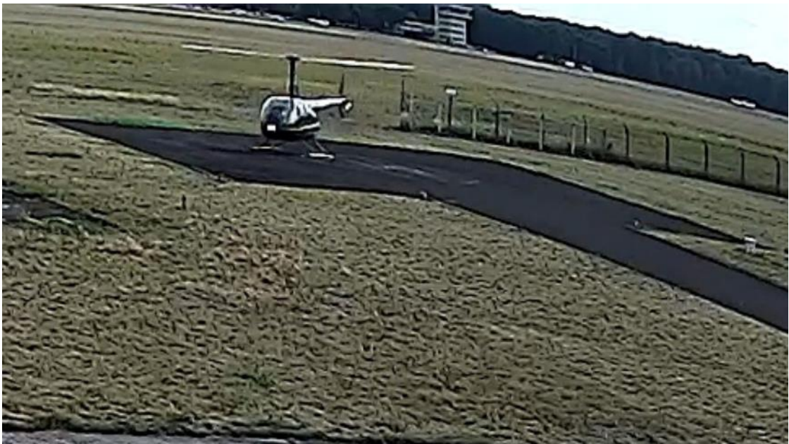
Figure 8. Leftward rotation of approximately 315^\circ with simultaneous backward tilt [source: CCTV footage].
