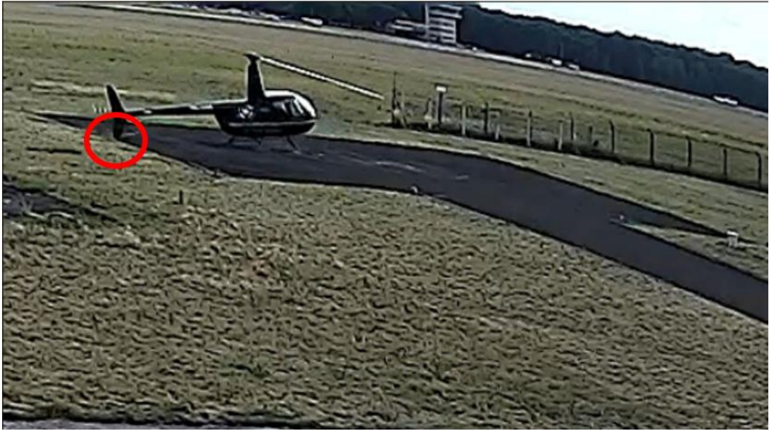
Figure 9. After another rotation of approximately 90^\circ with the tail skid hitting the helipad for the first time (marked with a red circle) [source: CCTV footage].
