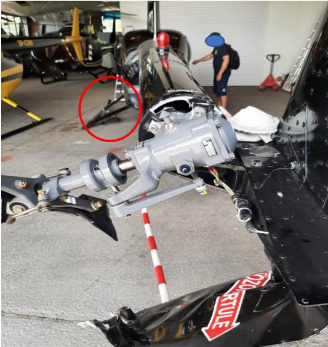
Figure 14. Broken angle gearbox including attachment to the tail boom assembly, damaged skid landing gear (red circle, left skid).
