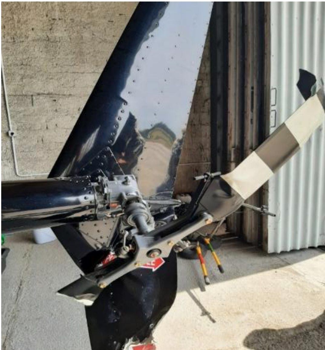
Figure 12. Destroyed tail rotor, damaged angle gearbox attachment to the tail boom.
