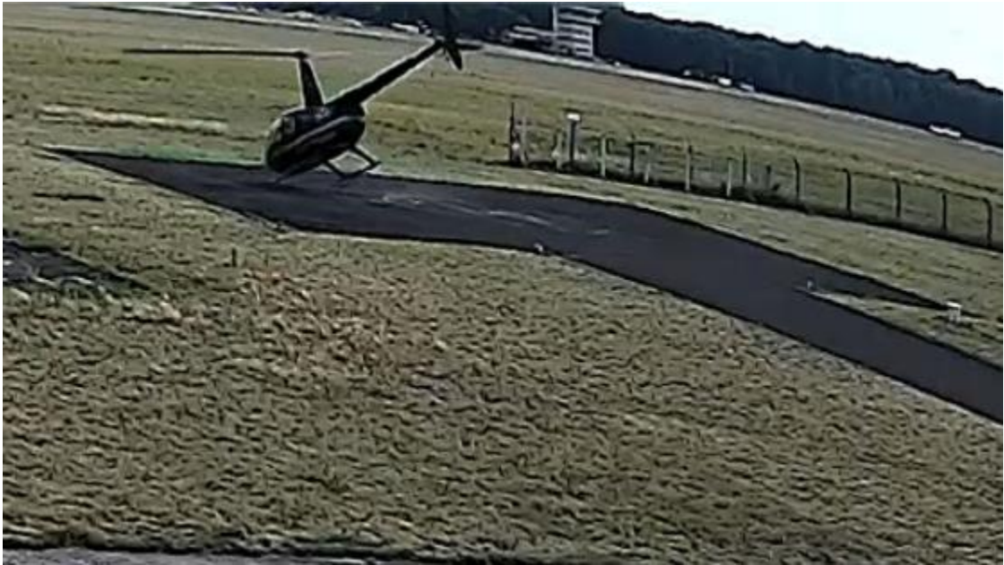
Figure 7. Leftward rotation of approximately 180^\circ with simultaneous forward tilt [source: CCTV recording].
