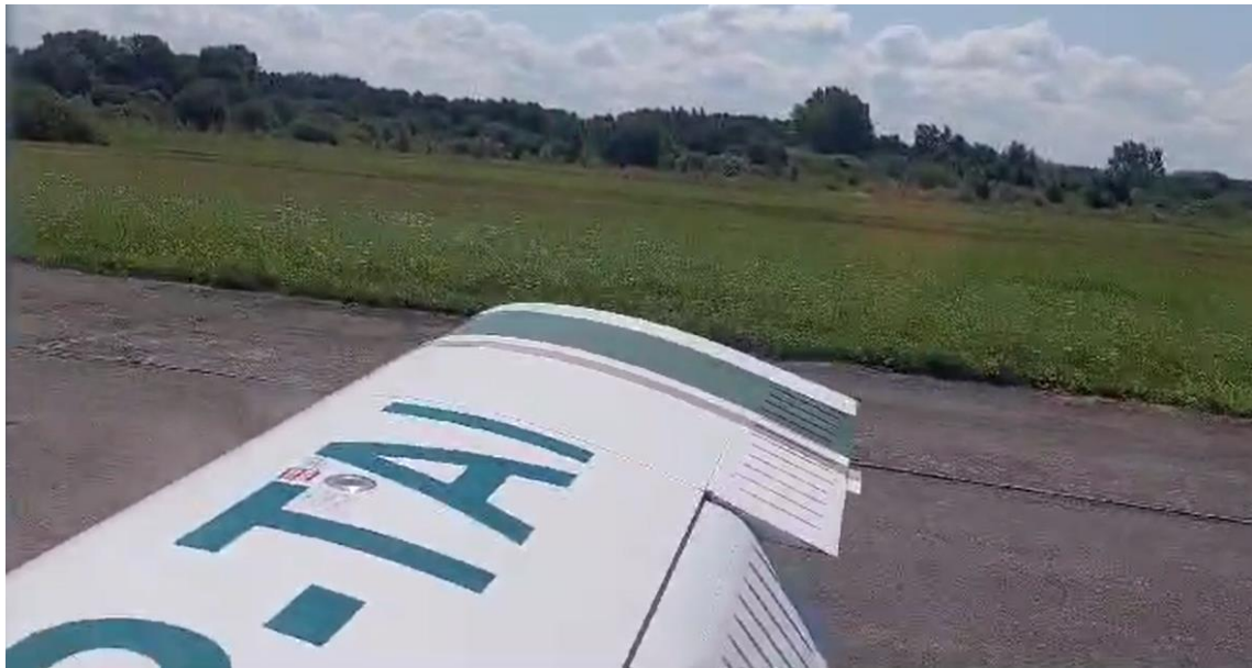
Fig. 2. Visible flaps deflected into the landing position [source: passenger]
