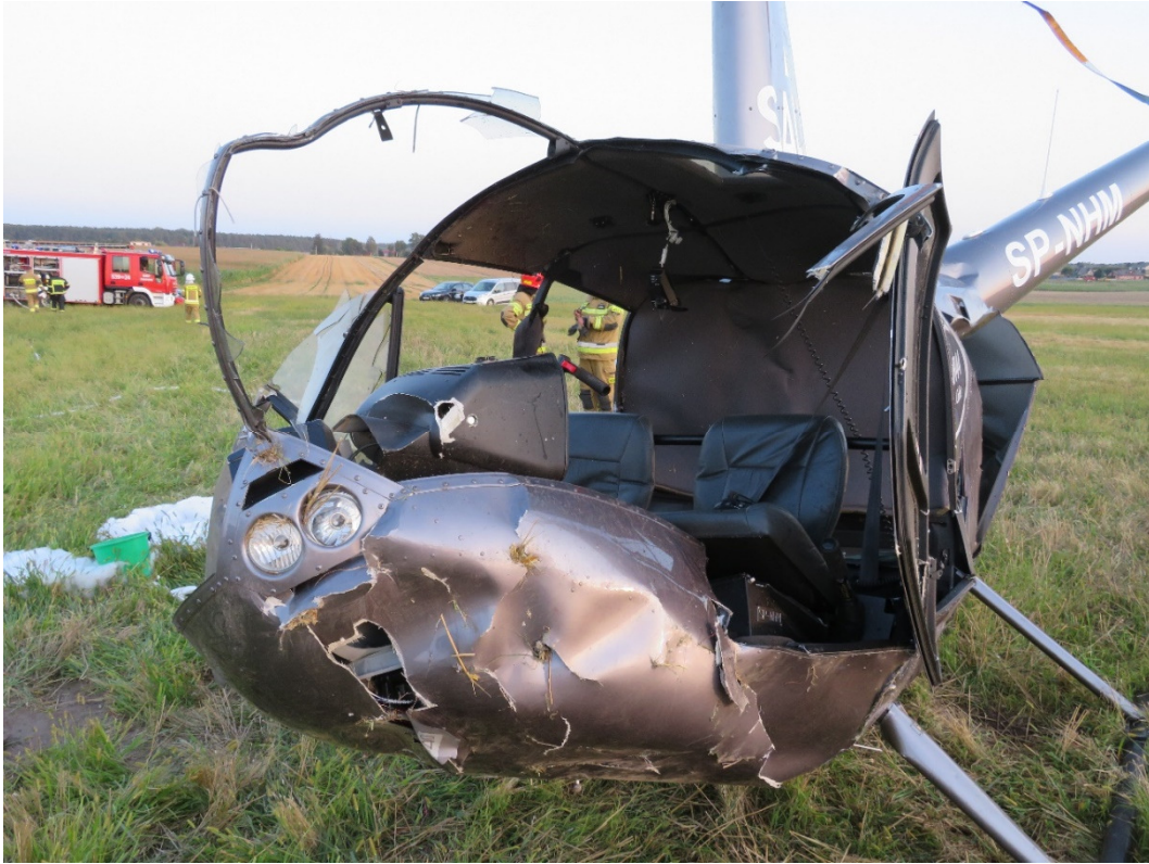
Fig. 6. Deformed left side of the helicopter cabin
