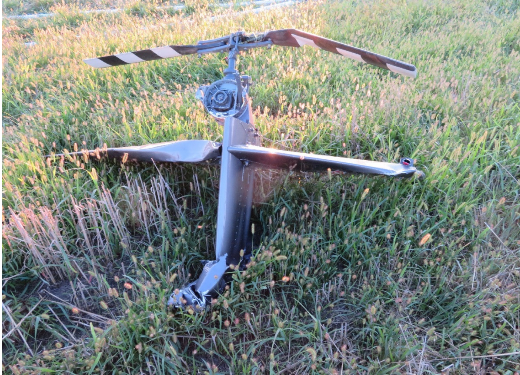
Fig. 3. Part of the tail boom with final drive and tail rotor
