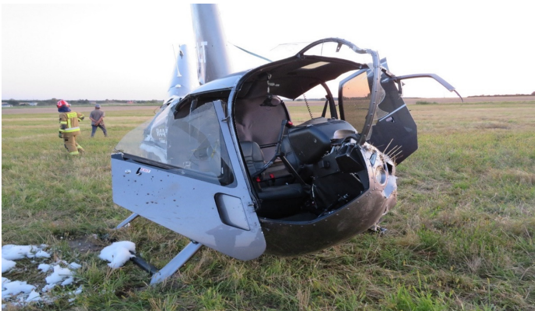
Fig. 5. Deformed right side of the helicopter cabin
