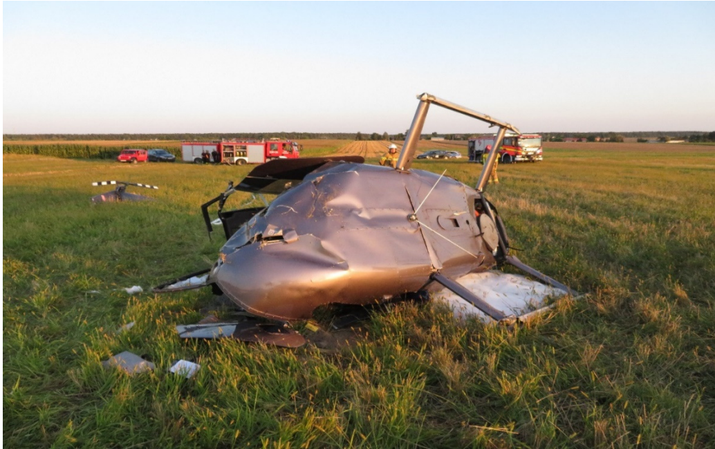
Fig. 4. Visibly damaged lower part of the fuselage
