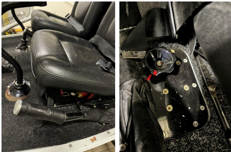
Fig. 4. The collective (on the left) and the lock knob (on the right)
