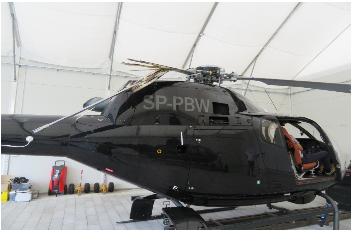
Fig. 5. Damage to the main rotor hub, main rotor blades and fuselage.
