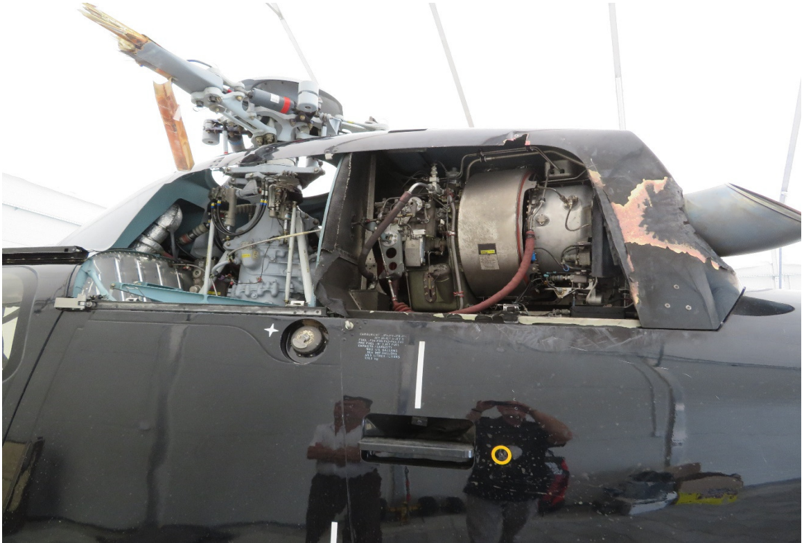
Fig. 6. Visible thermal changes on the fuselage after the hot engine start.
