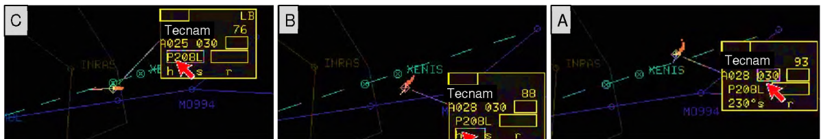
Fig. 2. Screenshots of PEGASUS_21 system at the APP ATC workplace at the time of: A - change the heading to 230°, B - instruction to change heading to 280°, C - confirmation of stabilisation according to VOR, [source: PANSAs]
