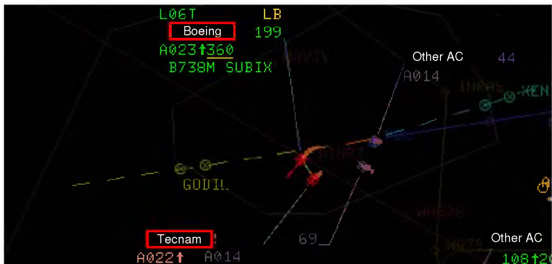
Fig. 3. Screenshots of PEGASUS_21 system at the APP ATC workplace during the proximity of Tecnam and Boeing aircraft (aircraft descriptions changed) [source: PANSA]
