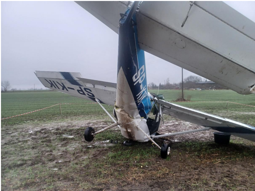
Rys. 5. Bending of the fuselage seeing from the compressed (crumpled) side. Notice the broken down leg of front landing gear below the fuselage and damaged mounting of the starboard wing.
