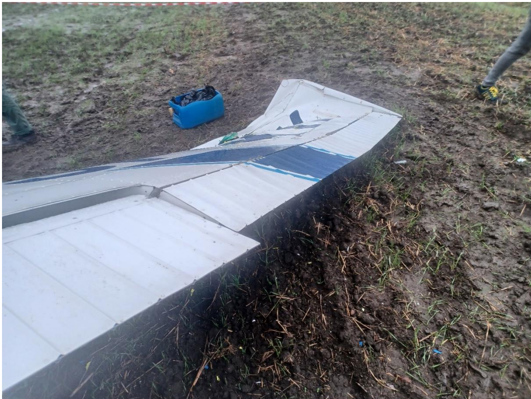
Rys. 3. Bending the outer part of the starboard wing (about \frac{1}{2} of the aileron span), from the leading edge
