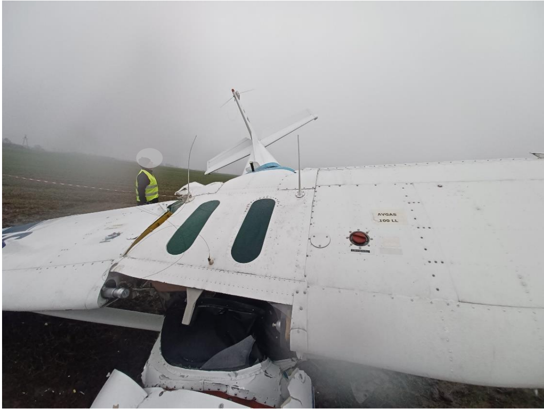
Rys. 2. Damage of the starboard wing fittings
