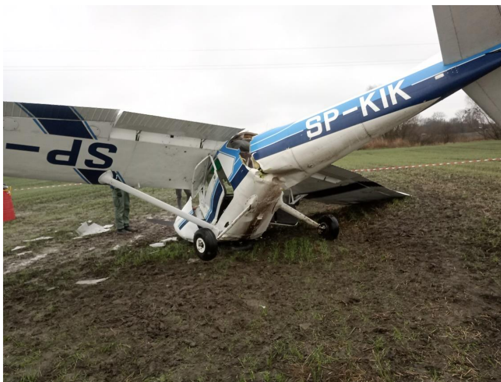
Rys. 1. Breaking of the fuselage behind the cockpit
