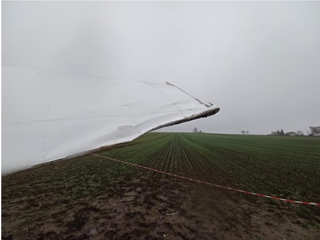
Rys. 4. Crumple of the port wing leading edge
