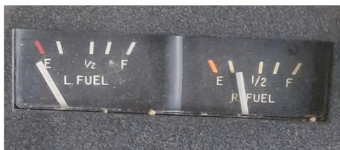
Fig. 2 Fuel gauge indications of the aircraft on 17 April 2025 (with electrical power on), after fuel tanks were emptied. [source: FDA]
