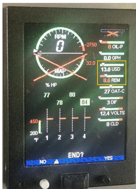
Fig. 3 EDM display indications (the remaining 8.6 gal of fuel is highlighted in orange) [source: FDA]
