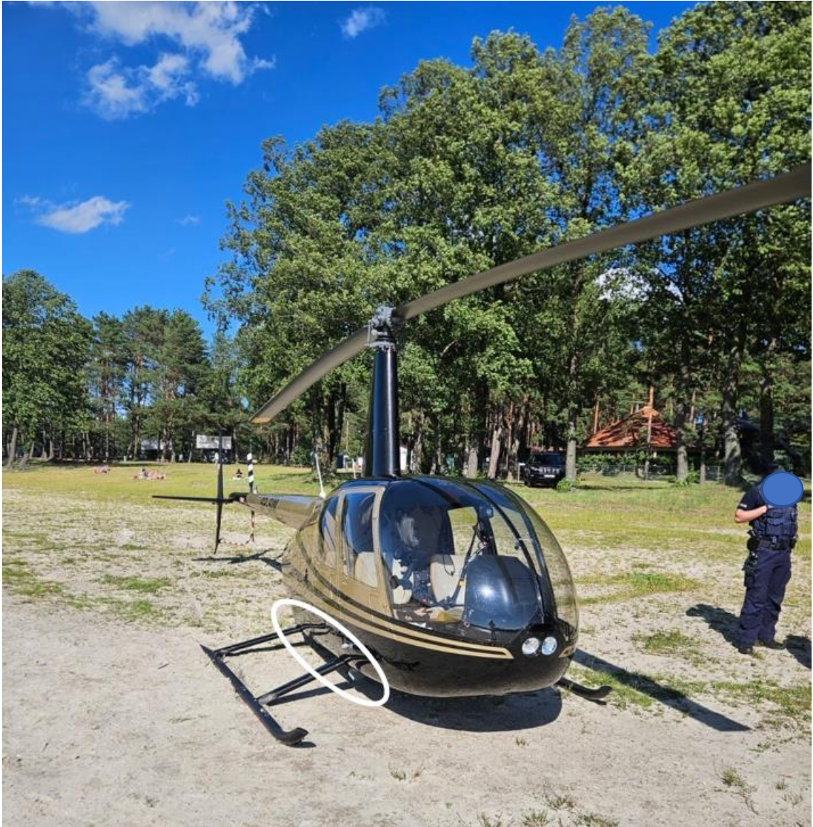
Fig. 3. Visible damage to the skid landing gear (left and right side) [source: owner of the helicopter]
