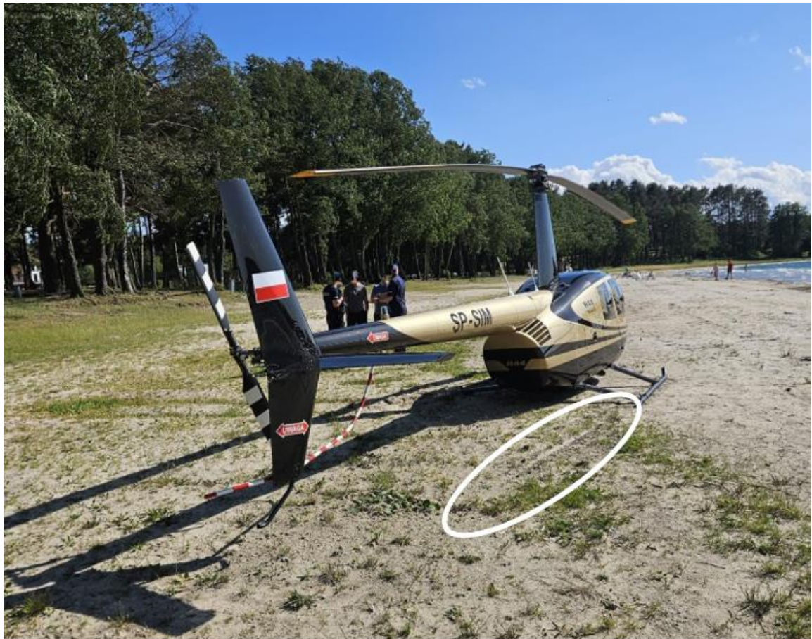
Fig. 2. The helicopter on the precautionary landing site – near hotel Warchoły, Świętajno Lake, touchdown coordinates 53°32'28" N, 20°48'08" E – the oval highlights the marks from the hard landing [source: owner of the helicopter]
