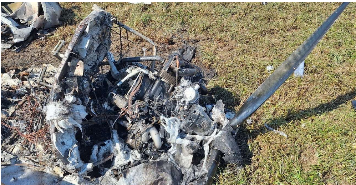
Fig. 7 Condition of the power unit – firewall, mount and engine detached, hub with two remaining blades. The white fabric is the remnant of a completely burnt engine cowling [source: PKBWL].
