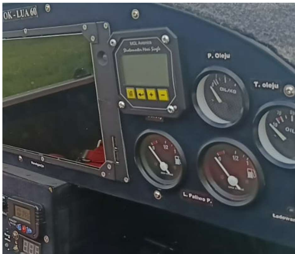
Fig. 15 Probable configuration of engine instruments [source: PKBWL].
