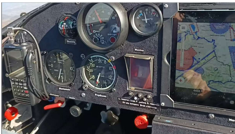
Fig. 14 Probable pilot instrument configuration in the Zodiac OK-LUA60 aircraft [source: PKBWL].
