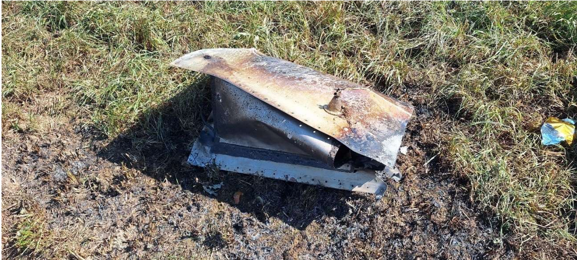
Fig. 6 Fuel tank torn from left wing caisson [source: PKBWL].
