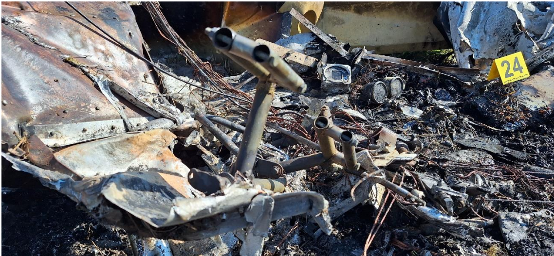
Fig. 9 Remains of the aircraft cabin – among others, visible rudder pedals and a few flight instruments [source: PKBWL].
