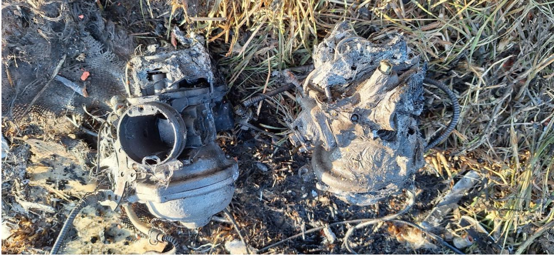
Fig. 8 Condition of the carburetors found in the wreckage, partially melted by the high temperature [source: PKBWL].
