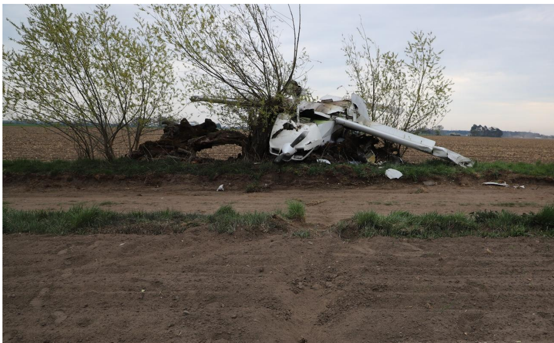
Figure 3. TB-9, D-EUGA aircraft after the crash. In front of the fuselage a mark of ground hit is visible.
