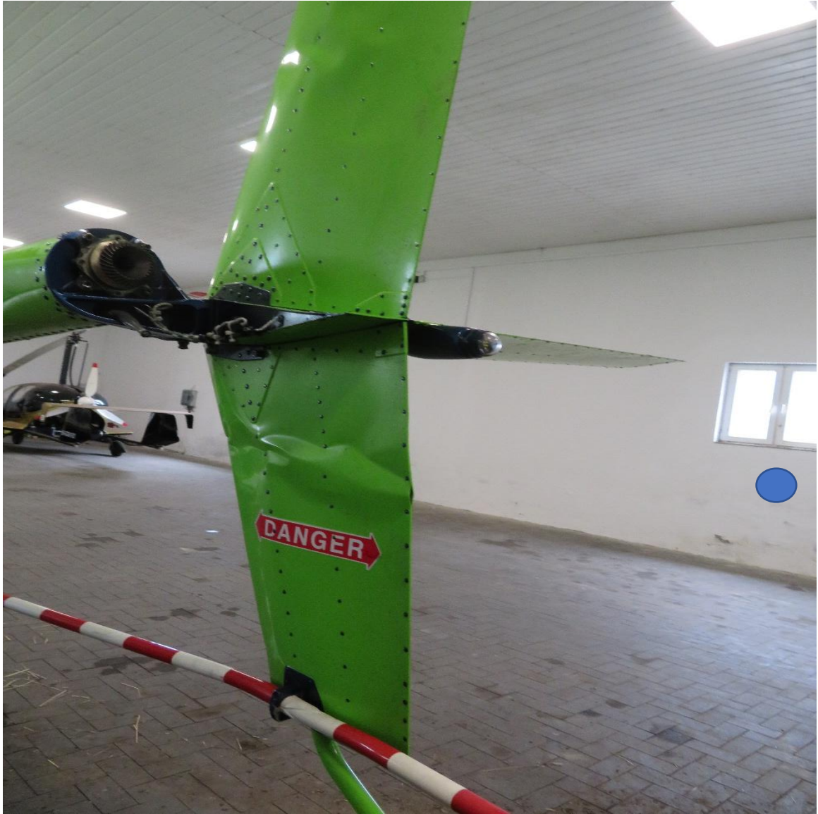
Fig. 3. Visibly missing tail rotor and tail gearbox [source: PKBWL].
