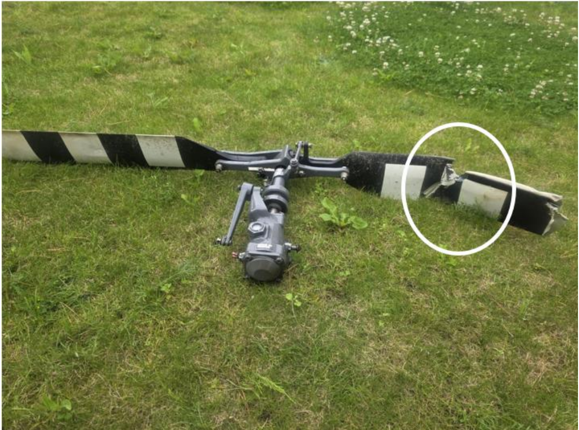
Fig. 5. Detached tail rotor along with angle gearbox. White colour shows the point where the tail rotor blade struck and severed another high-voltage power line [source: PKBWL].
